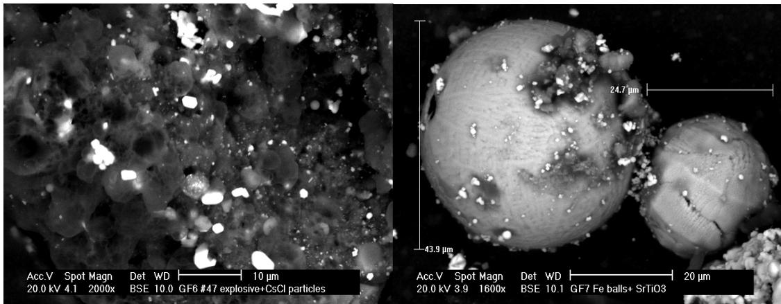
Fig. 1: SEM pictures of smear samples collected from a GZ point of two tests where stable CsCl and SrTiO<sub>3</sub> simulant sources were dispersed in “dirty bomb” like event.
