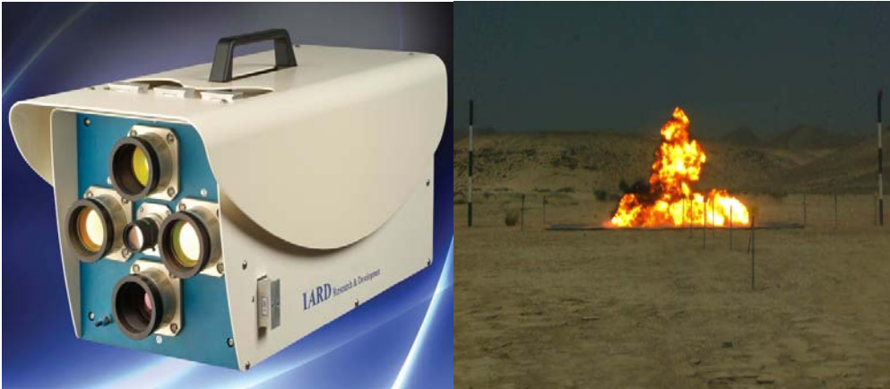
Figure 1: The ColoRad C7 (left) and high speed fireball snapshot 10 ms following TNT detonation (right).
