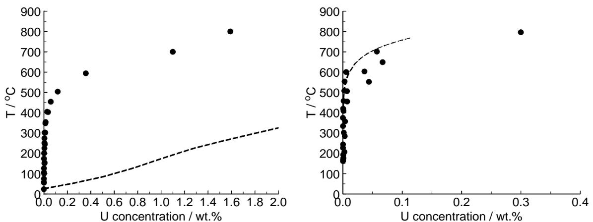
Fig. 1. Solubility of uranium in liquid gallium (left) and indium (right). Symbols show experimental data obtained in the present work, lines – proposed liquidus lines in U-Ga and U-In binary systems [1].
