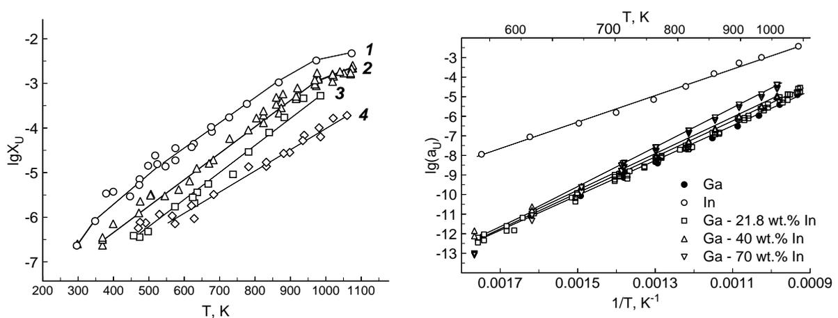
Fig. 2. Solubility of uranium in liquid gallium (1) and Ga-In alloys (2–4). Indium content of the alloys, wt.%: 21.8 (2), 40 (3), 70 (4). Fig. 3. Activity of uranium in liquid gallium, indium and Ga-In alloys (composition is shown for each set of data)
