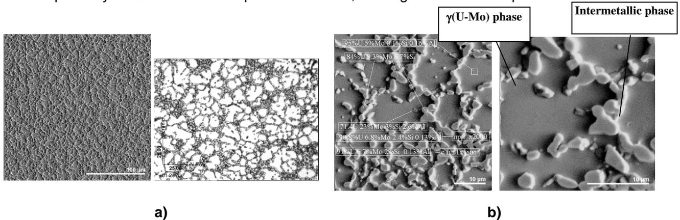
Fig.1. Structures of alloyed UMo two-phase alloy; a – U + 5.7Mo + 0.9Si; b – U + 6.3Mo + 0.9Si + 0.15Al.
