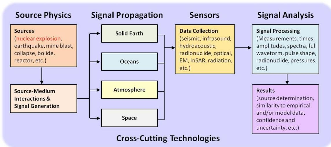
Figure 2. Representation of ground-based nuclear explosion monitoring elements.
