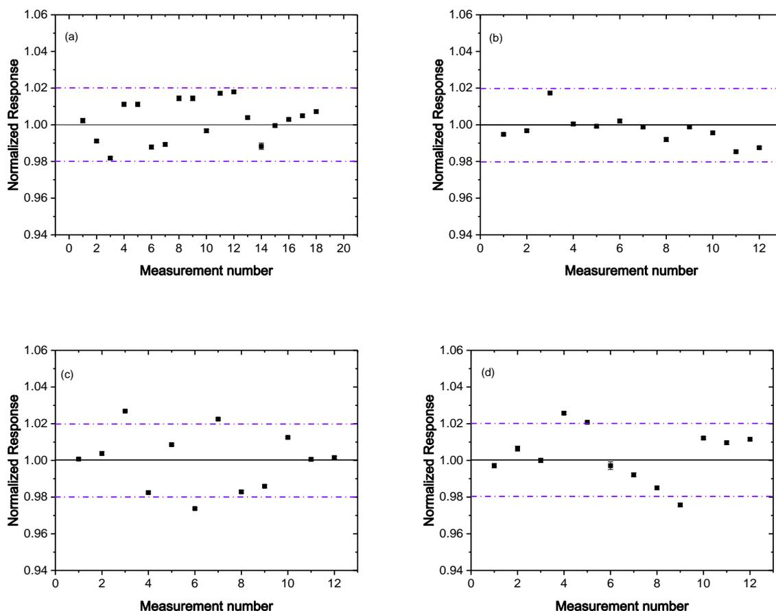
**Figure 1: Stability test for the ionization chambers with their sensitive volume lengths of: (a) (Commercial ionization chamber Victoreen) 10 cm; and homemade ionization chambers (b) 10 cm; (c) 3 cm and (d) 1 cm. The maximum uncertainty of the measurements in Figures a, b, c and d was 0.17 %, not visible on the graphs.**
