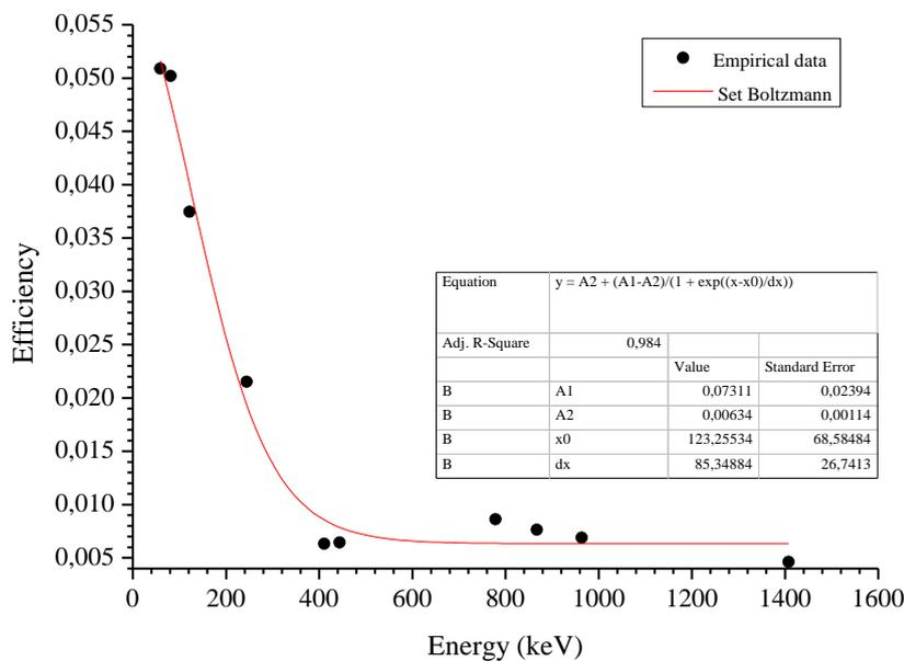
**Figure 2: Measurement System efficiency curve.**
