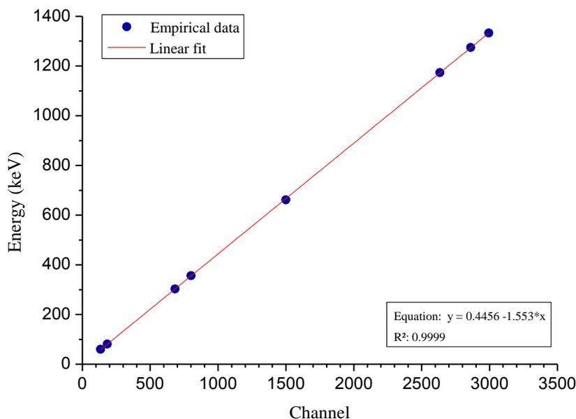
**Figure 1: Measurement System straight calibration.**
