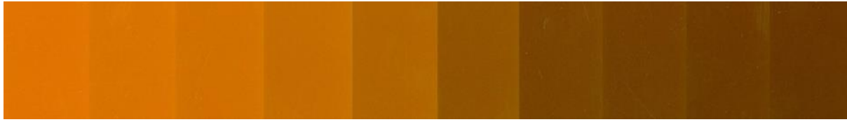
Figure 3: Darkening degree sequence of the strips after irradiation with the following doses: 0 (non-irradiated); 0.25; 0.50; 1.00; 2.00; 5.00; 10.0; 12.0; 15.0 and 18.0 cGy.
