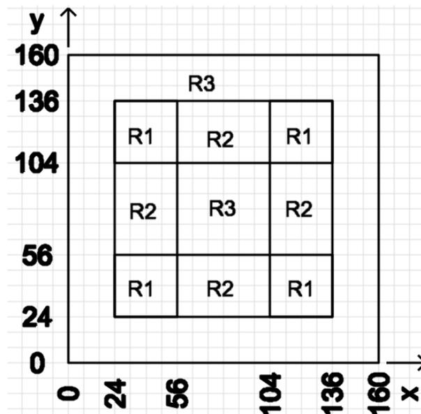
**Figure 1: Geometry, in cm.**
