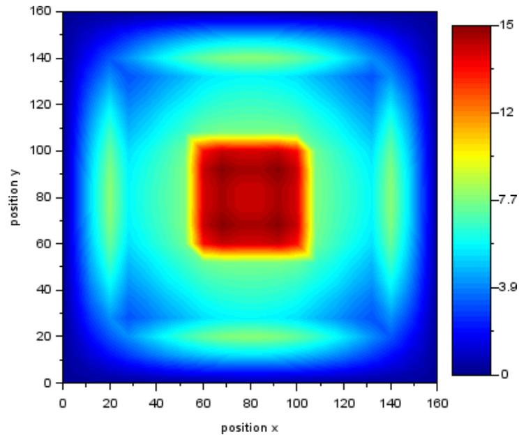
Figure 3: Thermal neutron scalar flux in  $cm^{-2}s^{-1}$ .
