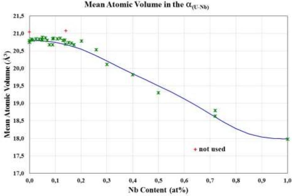
**Figure 3: Mean atomic volume in the  $\alpha$ -phase U-Nb System**
