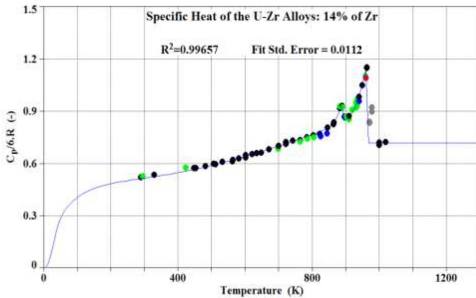
Figure 5: Data reduction of the specific heat of the U-14%Zr alloy [56]
