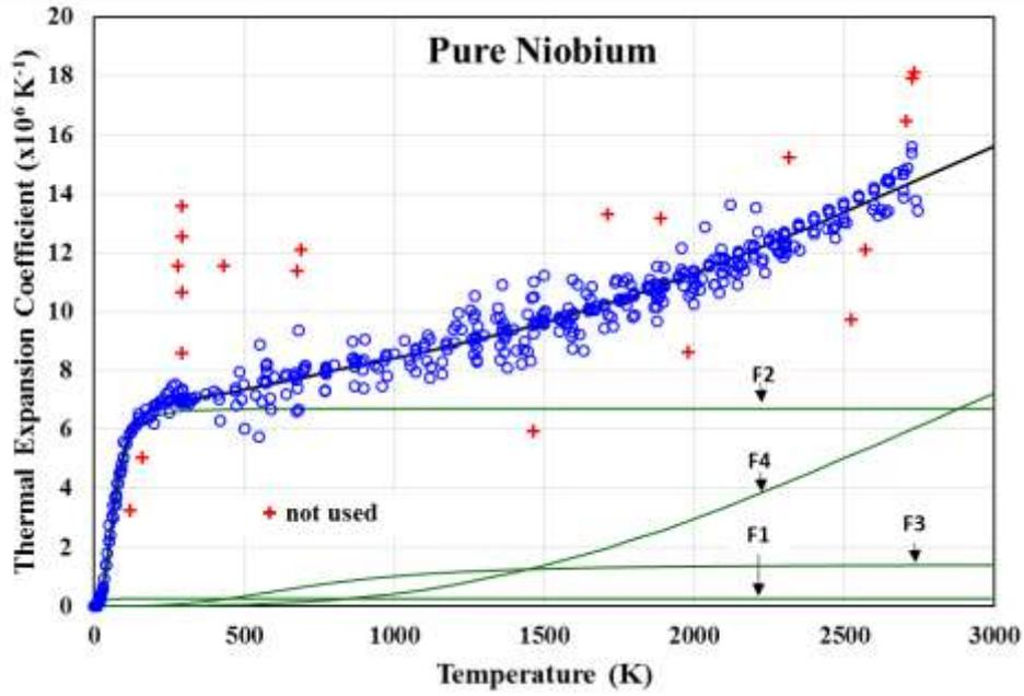
Figure 4: Data reduction of the linear thermal expansion coefficient of the pure Niobium
