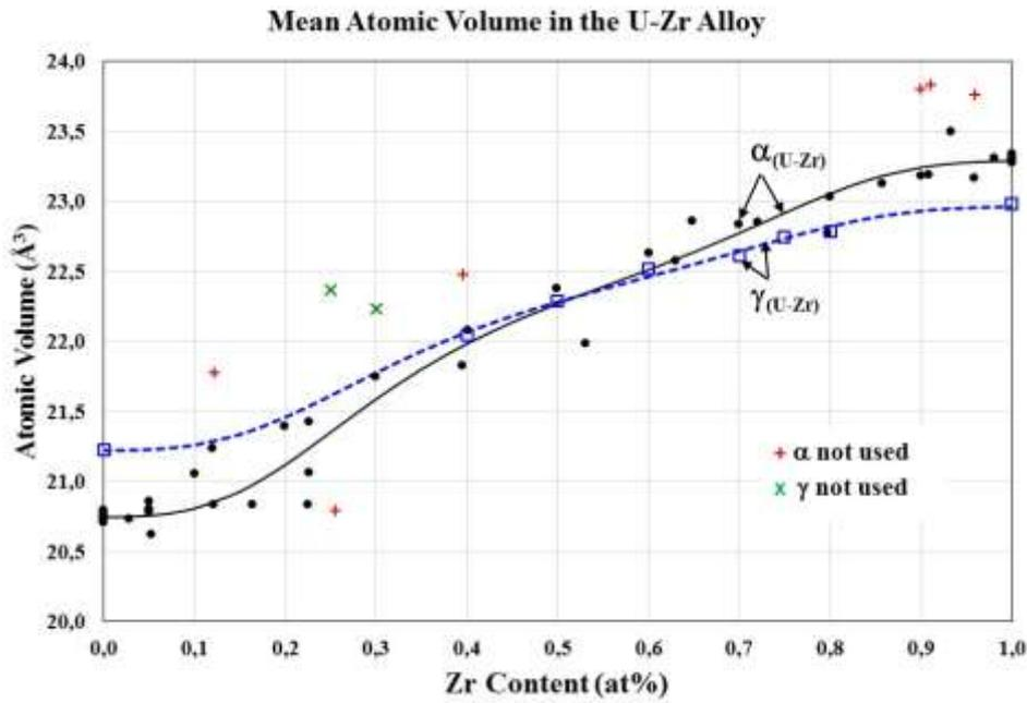
**Figure 2: Mean atomic volume in the  $\alpha$ - and  $\gamma$ -phases of the U-Zr Systems**
