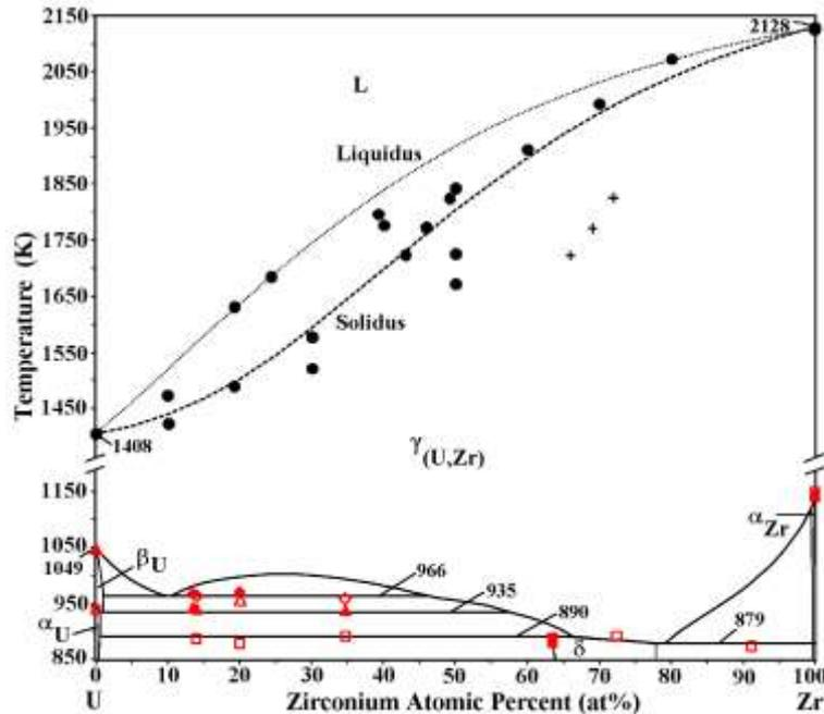
Figure 1: Phase diagram of the Uranium-Zirconium System [23].
