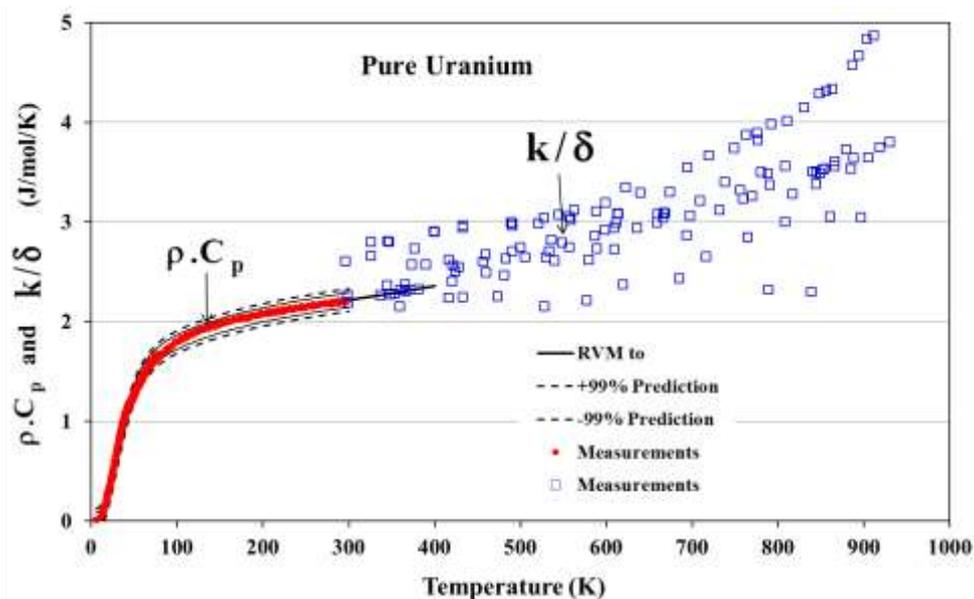
Figure 7:  $\rho \cdot C_p$  (low temperature) and  $k/\delta$  (high temperature) for pure Uranium [27]
