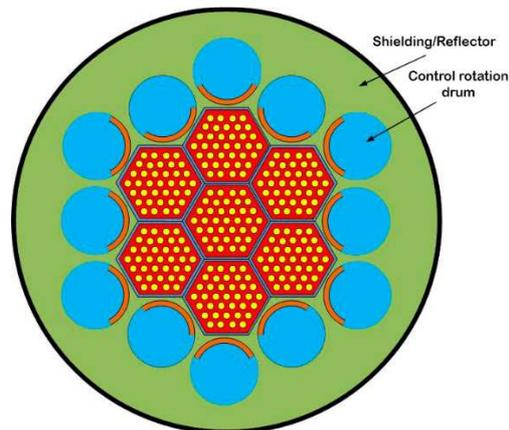
**Figure 1: Core concept proposed for the space nuclear microreactor.**
