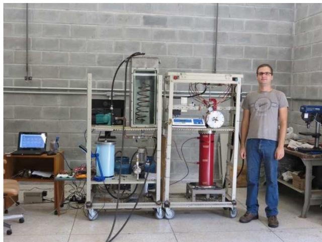
**Figure 8: Rankine work bench to test the Tesla turbine.**
