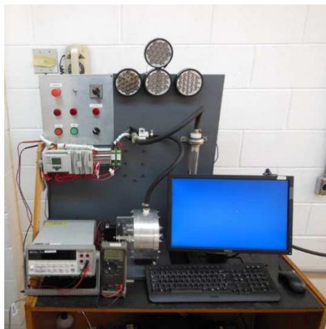
**Figure 9: Test of the Passive Multi Fluid Turbine (an evolution of the Tesla turbine).**
