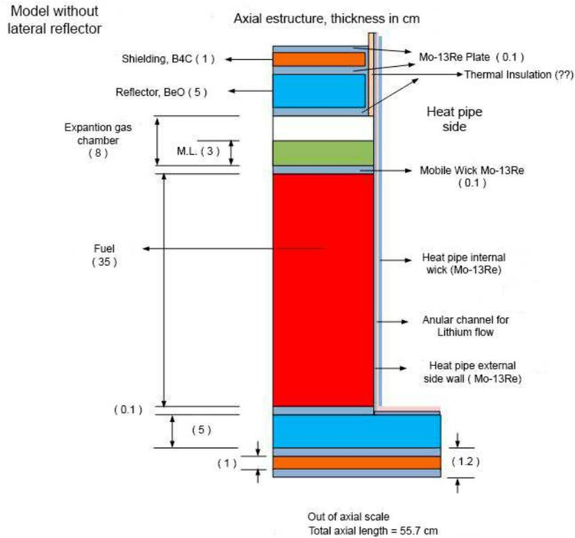
**Figure 2: Core concept proposed for the space nuclear microreactor.**
