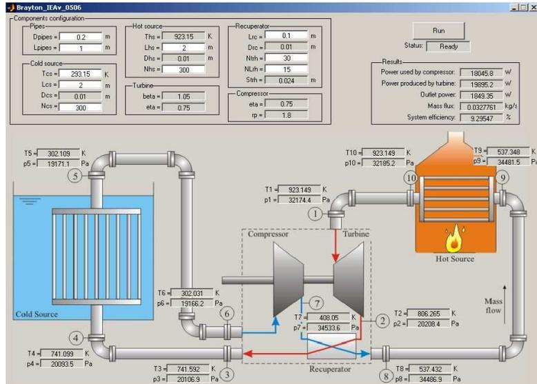
**Figure 3: Closed Brayton cycle, schematic view with temperature, pressure and flow steady state values.**
