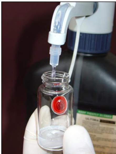
**Figure 1: Adding the Ultima Gold AB Packard cocktail to the scintillation vial**
