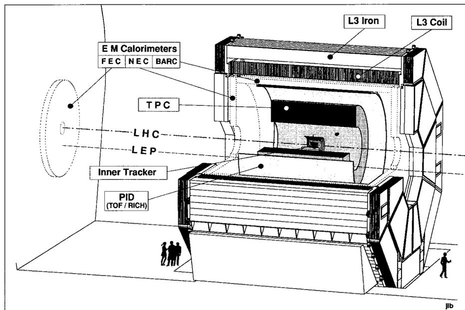
The proposed ALICE detector to study heavy ion collisions in the LHC ring to be built in CERN's 27-kilometre LEP tunnel.
