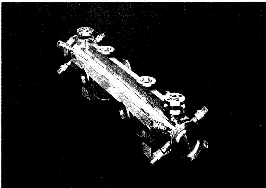
drive linac power source. The high frequency allows the high accelerating gradient of 80 MV/m, resulting in a collider 2x4 km long for 500 GeV collision energy and 2x16 km long for 2 TeV. The drive linac power source eliminates the need for large numbers of klystrons, so most of the accelerator tunnel will be empty of active radiofrequency elements.
