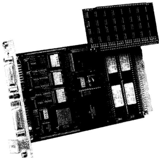
The VM30 is a single-height, general purpose, triple processor CPU board with up to 10 MIPS performance. The VM30 provides multiprocessing power and multi-tasking capability, fully equal to many dual-height solutions.
