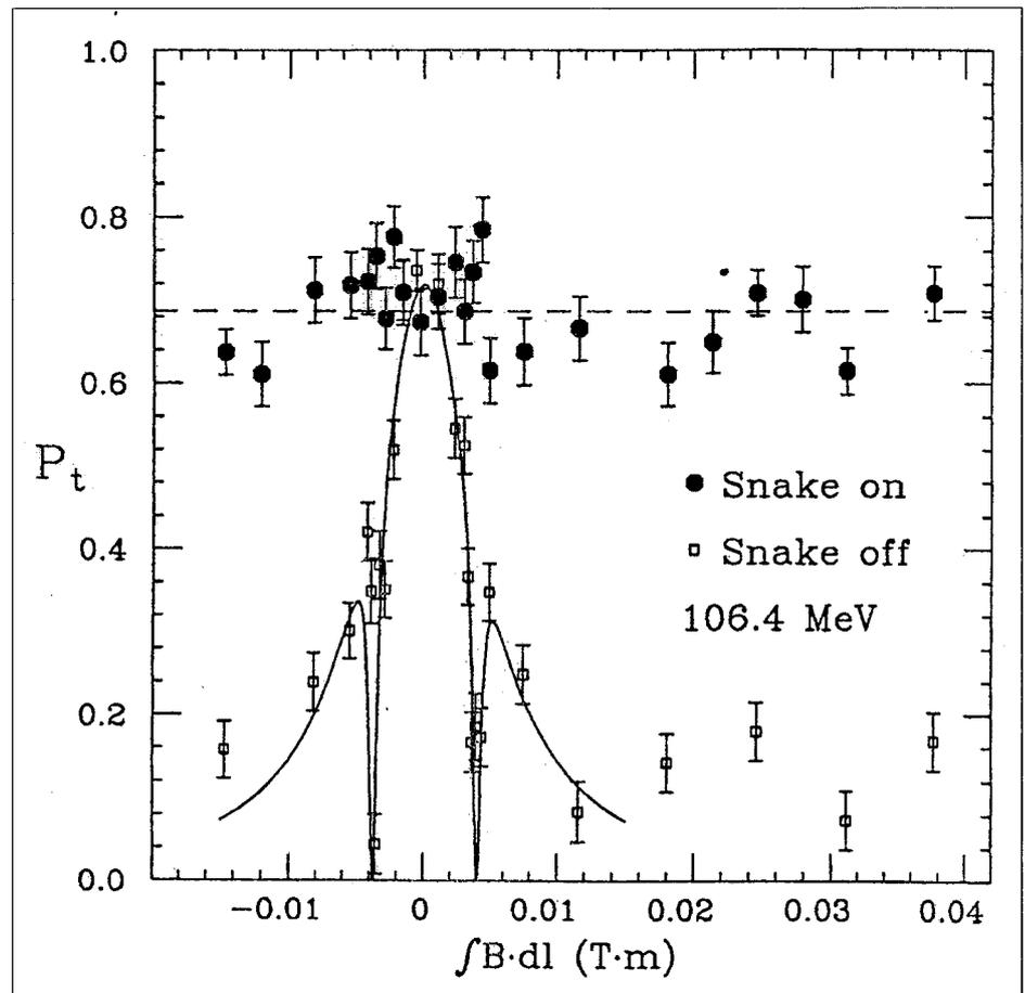
'Siberian Snakes' save spin. The total transverse proton beam polarization at the Indiana Cooler Ring plotted against the imperfection magnetic field integral with the Siberian snake device on (circles) and off (squares). The solid line is a fit to the imperfection depolarizing resonance peak and radiofrequency resonance dips; the dashed line is a constant fit to the snake-on data.
