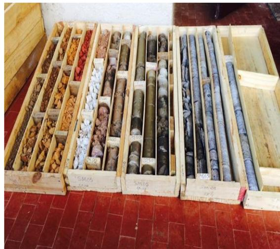
**Figure 5. Typical soil composition, from top sandy clay to gneissic rock**
