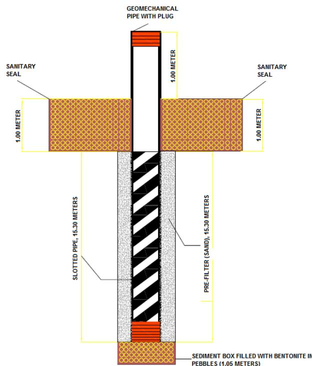
**Figure 6. Monitoring well arrangement**
