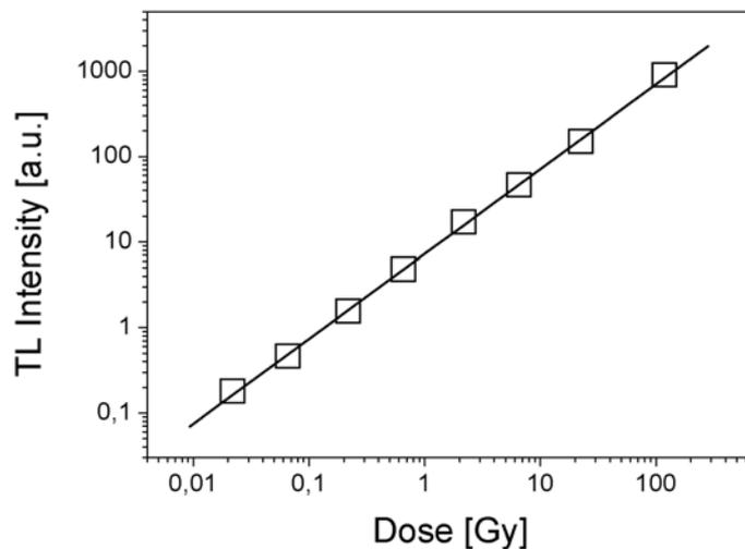
Figure 7. Dose response of  $\text{Li}_2\text{B}_4\text{O}_7:\text{Cu}$  (0.5 wt %) between 0.01 and 100 Gy. The solid line is a linear fit included for the eye guide.
