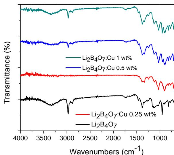
Figure 2. The FT-IR-ATR spectra of blank lithium tetraborate and lithium tetraborate doped with copper (0.25, 0.5, and 1.0 wt %).
