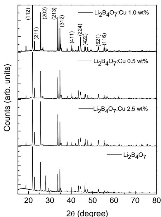
Figure 1. X-ray diffraction pattern of undoped lithium tetraborate and lithium tetraborate doped with copper (0.25, 0.5, and 1.0 wt %).
