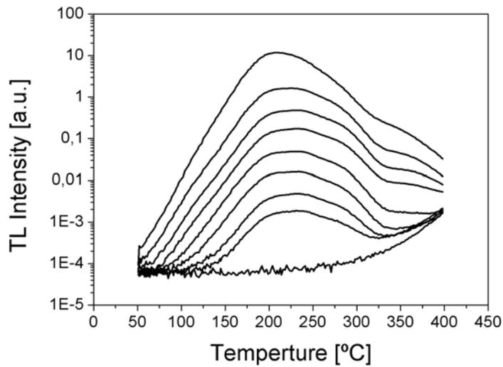
Figure 6. Glow curves of  $\text{Li}_2\text{B}_4\text{O}_7:\text{Cu}$  (0.5 wt %) from 100 up to 0.01 Gy from top to bottom, respectively. The bottom curve has been recorded for an unirradiated sample.
