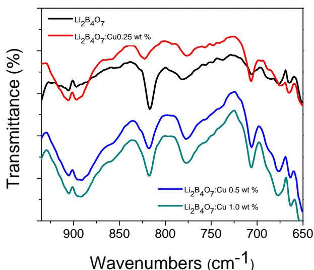
Figure 3. The FT-IR-ATR spectra of Li<sub>2</sub>B<sub>4</sub>O<sub>7</sub> and Li<sub>2</sub>B<sub>4</sub>O<sub>7</sub>:Cu doped with 0.25, 0.5, and 1.0 wt %.
