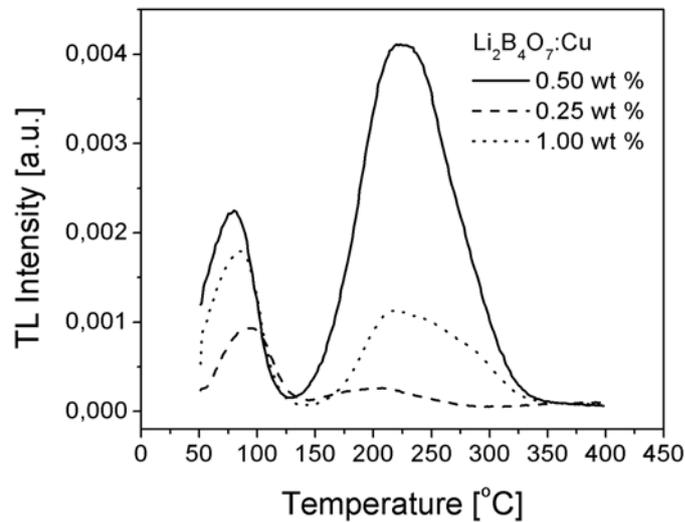
Figure 4. TL glow curves of  $\text{Li}_2\text{B}_4\text{O}_7$  doped with different concentration of copper.
