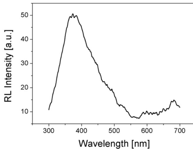
Figure 10. RL spectrum of  $\text{Li}_2\text{B}_4\text{O}_7:\text{Cu}$  (0.5 wt %).
