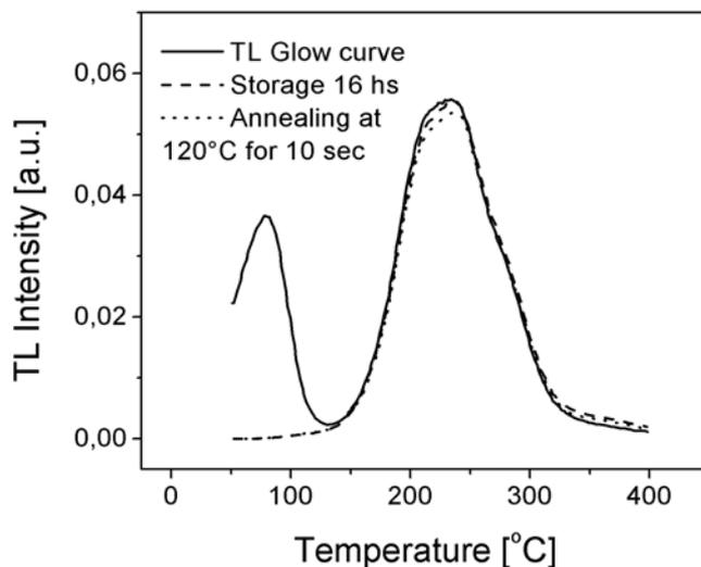
Figure 5. TL glow curve of  $\text{Li}_2\text{B}_4\text{O}_7:\text{Cu}$  (0.5 wt %) measured immediately after irradiation (solid), after 16 hours of storage in darkness and at RT (dash) and after an annealing at  $120^\circ\text{C}$  for 10 seconds (dot), respectively.
