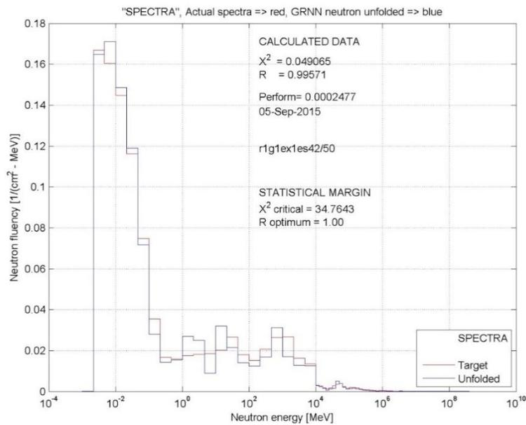
Figure 7. Best spectrum obtained at testing stage compared with target spectrum
