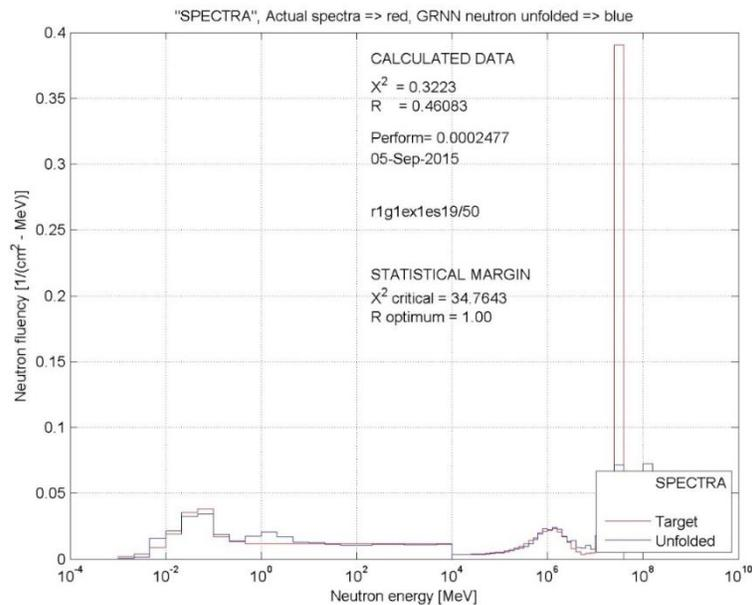
Figure 9. Worst spectrum obtained at testing stage compared with target spectrum
