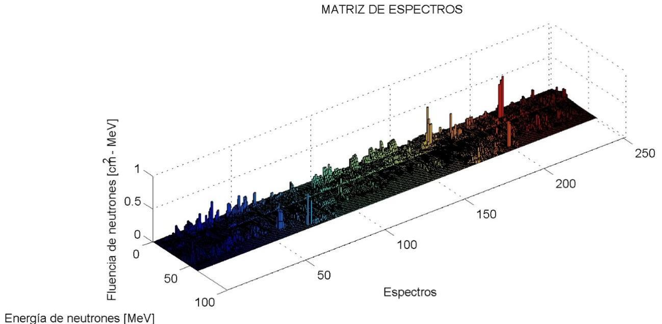
Figure 4. Neutron spectra data set, expressed in energy units, used to train the GRNN
