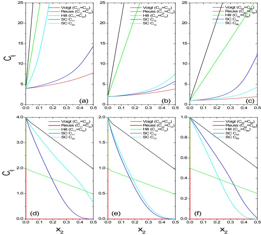
Upper row: case of hard phase #2, lower row: case of voided phase #2. a,d)  $C_{11}, C_{22}, C_{33}$ , b,e),  $C_{12}, C_{13}, C_{23}$  and c,f)  $C_{44}, C_{55}, C_{66}$ .
