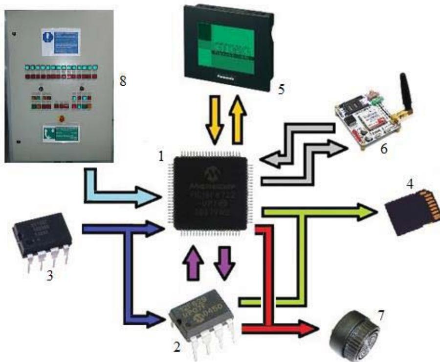
**Figure 2: Simplified diagram of Autonomous Monitoring Unit, where 1 is the Main Microcontroller, 2 Secondary Microcontroller, 3 Real Time Clock and Calendar, 4 Secure Digital Card Memory, 5 Man Machine Interface, 6 General Packet Radio Services Module, 7 Audible alarm and 8 Control Panel**
