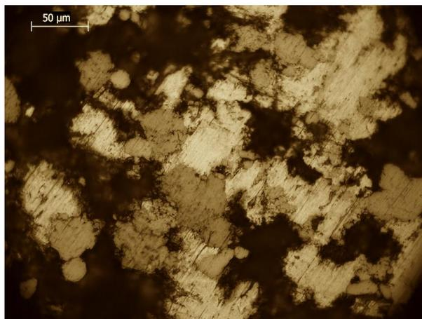
**Figure 3. Optical micrograph of sample 75W25Cu surface, at higher magnification, showing the W particles (median grey contrast), Cu particles (light gray contrast) and porosity (dark contrast). Not etched.**
