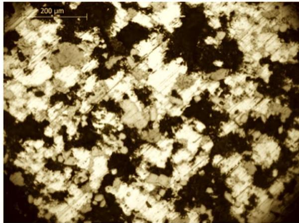
**Figure 2. Optical micrograph of sample 75W25Cu surface, showing the W particles (median grey contrast), Cu particles (light gray contrast) and porosity (dark contrast). Not etched.**
