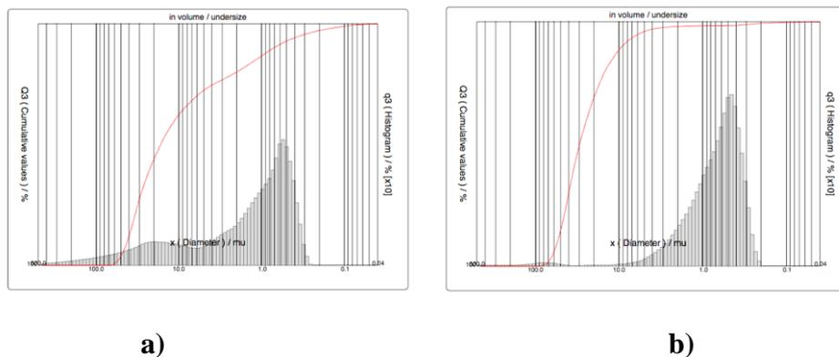
**Figure 1. Particle size distribution for the used (a) tungsten and (b) copper powders.**
