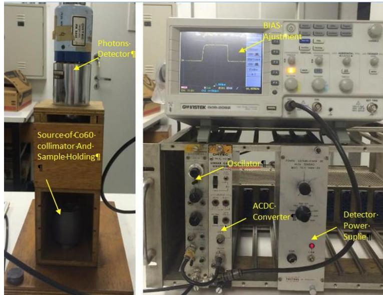
**Figure 5. Experimental set-up showing the main used equipments.**
