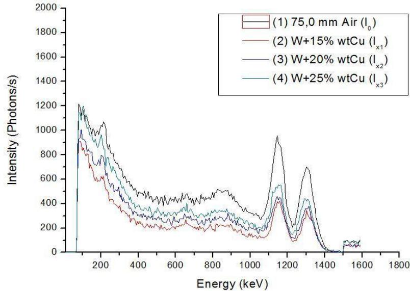
**Figure 7. Intensity absorption by percent amount of tungsten in the samples.**
