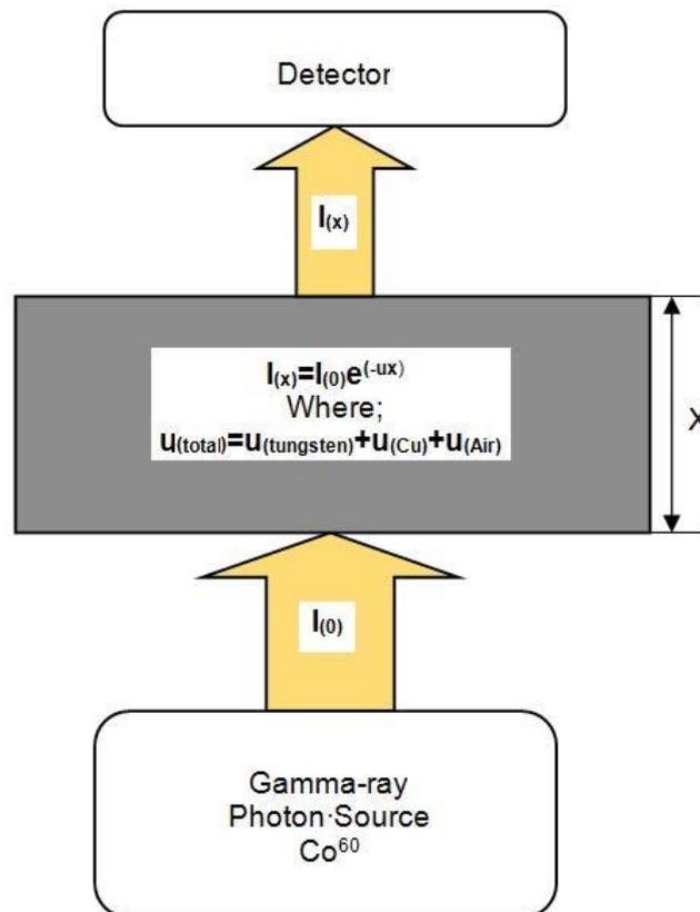
**Figure 4. Schematic set-up diagram for the linear attenuation coefficient measurement.**
