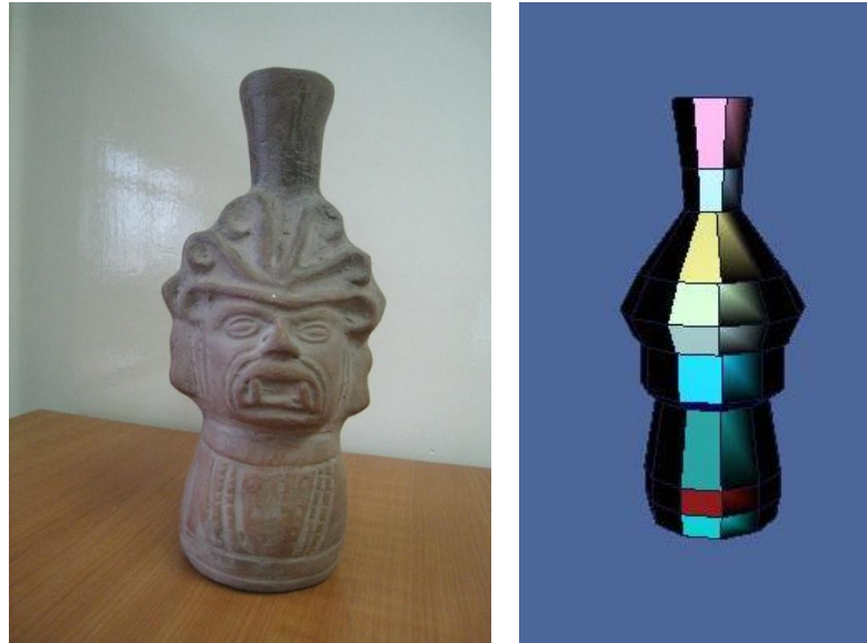
Figure 18 IPEN inter-comparison exercise sample and MCNP model
