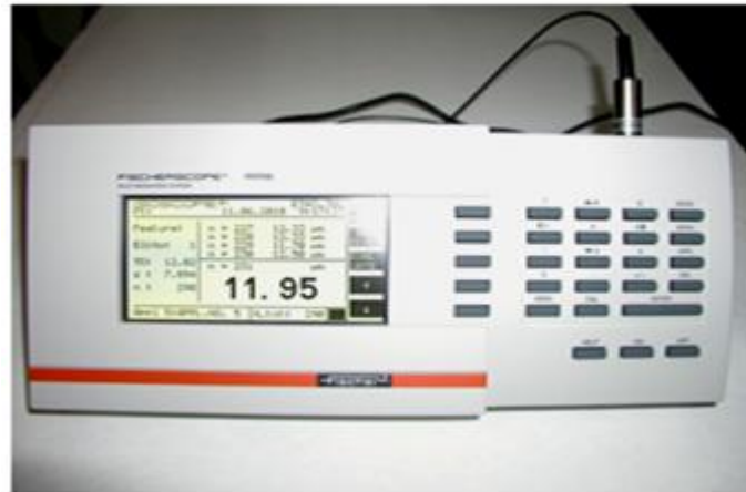
Figure 10 Device used to measure the thickness of the oxide
