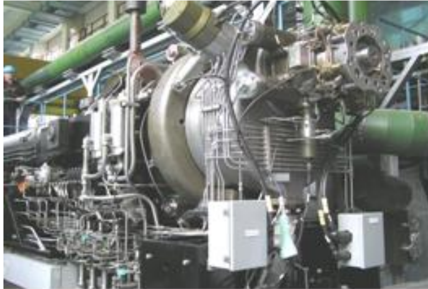
Figure 1 CANDU 600 Fuelling Machine (partial view)
