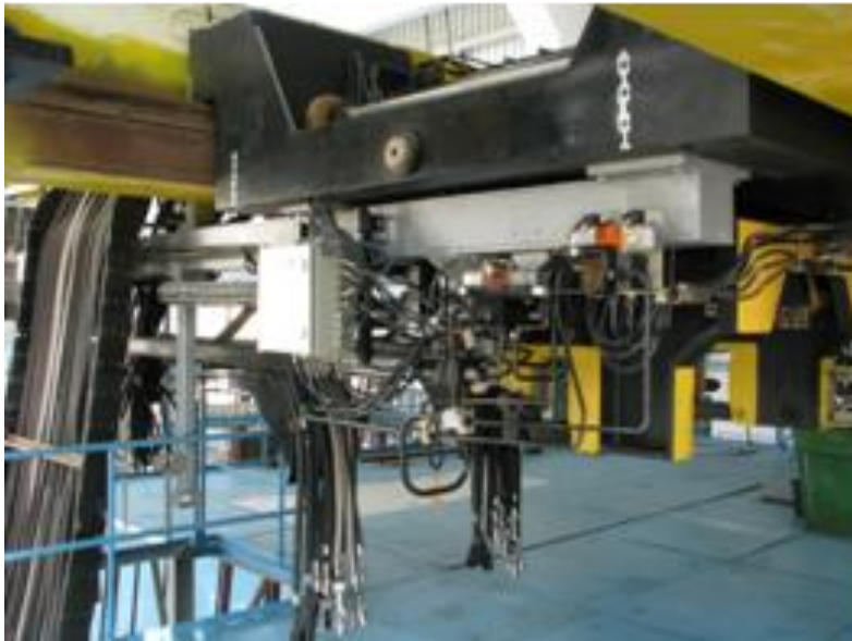
Figure 4 F/M testing rig: bridge, carriage and catenary (partial view)
