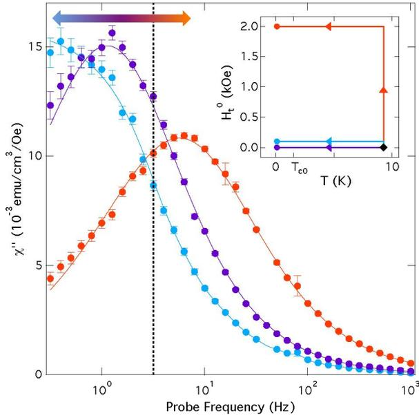
**Fig. 2:** Contrasting response of the imaginary part of the susceptibility to small and large transverse fields (inset) after cooling in a constant energy configuration. The shift down in frequency is unexpected, indicating collective behavior of hundreds of spins transiting the free energy surface and changing the system's ground state. At large transverse fields, tunneling probabilities are enhanced and the spectrum moves to higher frequency [Following Ref. 1].
