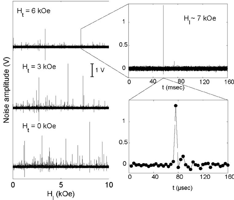
**Fig. 6:** Barkhausen noise recorded on sweeping the longitudinal magnetic field through a hysteresis loop in the ferromagnet  $\text{Nd}_2\text{Fe}_{14}\text{B}$ . All data are taken at fixed temperature. The noise decreases with increasing transverse magnetic field as the transverse field induces local random magnetic fields that pin the domains. The ability to alter the pinning potential in this manner may have applications in magnetic storage [From Ref. 43].
