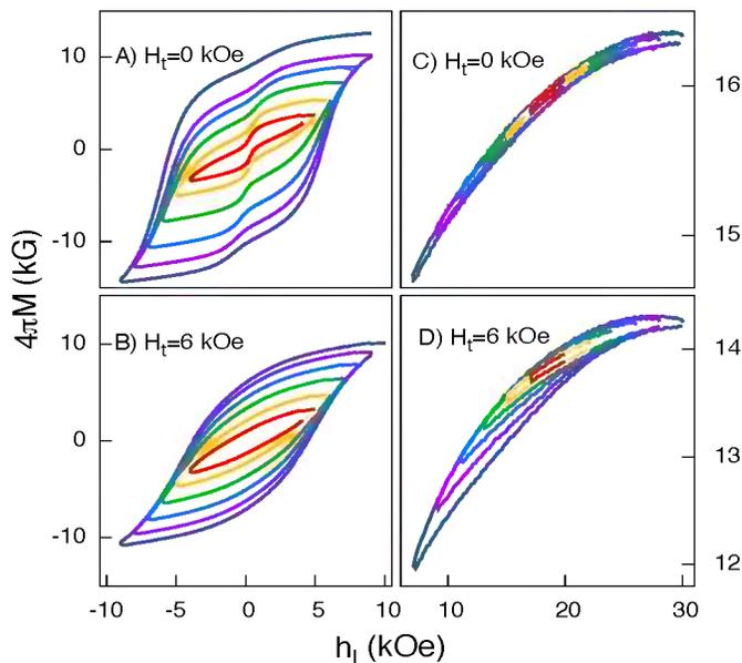
**Fig. 5:** Effects of transverse field on subloop evolution in the rare-earth ferromagnet  $\text{Nd}_2\text{Fe}_{14}\text{B}$ . (a,b) Nested subloops at low longitudinal field at room temperature. The subloops remain self similar in zero and 6 kOe of transverse field. (c,d) Nested subloops at high longitudinal field. Applying a transverse field *broadens* and *rotates* the subloops, destroying their self-similar nature [Following Ref. 39].
