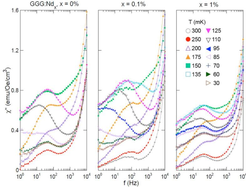
**Fig. 4:** The imaginary part of the ac magnetic susceptibility over 4 decades of frequency at milliKelvin temperatures for crystals of GGG with 0, 0.1% and 1% Nd doping. The disorder shifts and modulates the low frequency signatures of local magnetic order and spin cluster physics [From Ref. 29].
