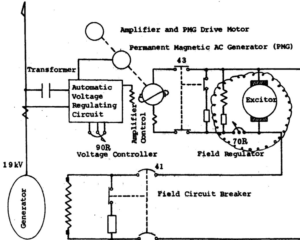
Figure 3-3 Improvement of Generator Field Regulator
