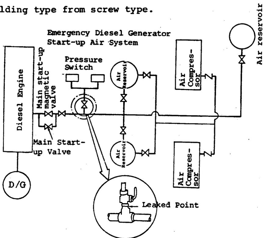
Figure 3-7 Repair on Emergency Diesel Generator
