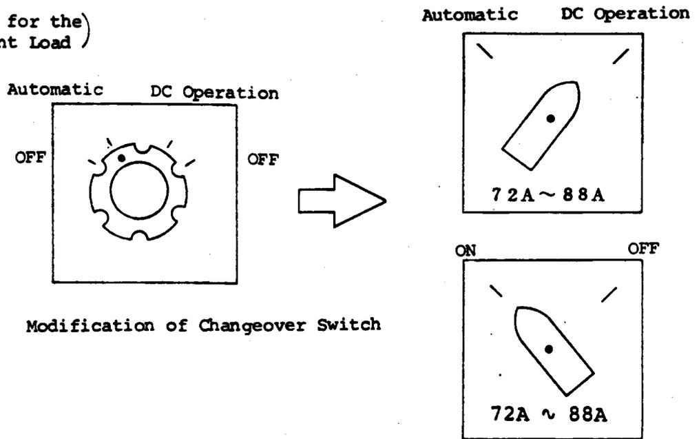
Figure 3-4 Example of Improvement of Vital Power Source Facility (1)
