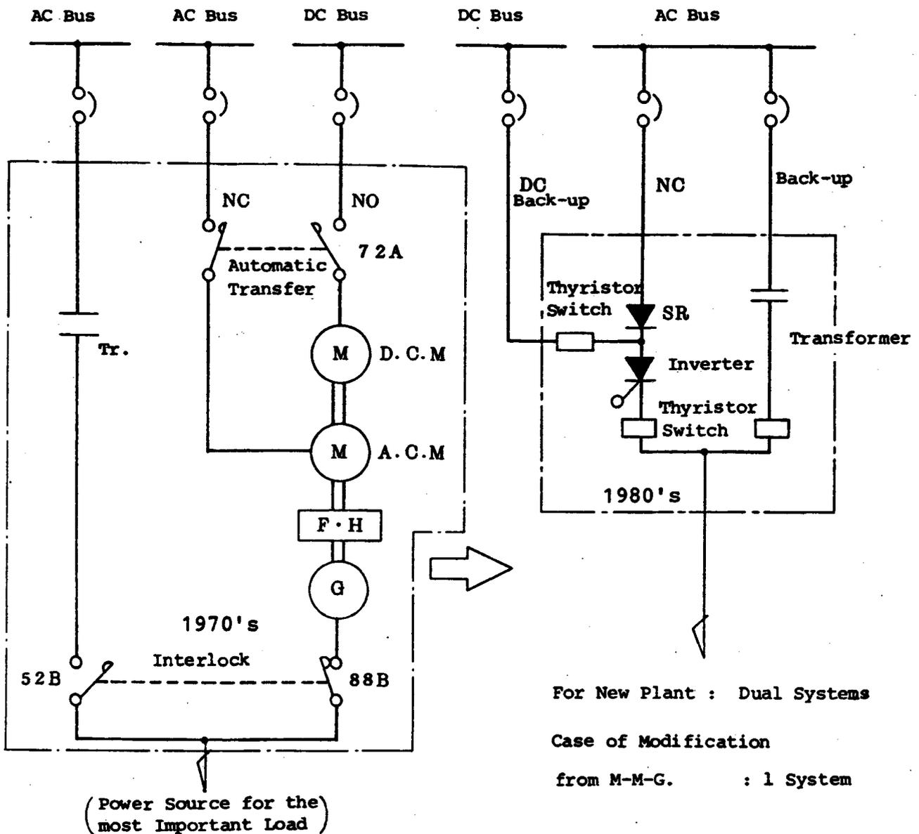
Figure 3-6 Example of Improvement of Vital Power Source Facility (3)
