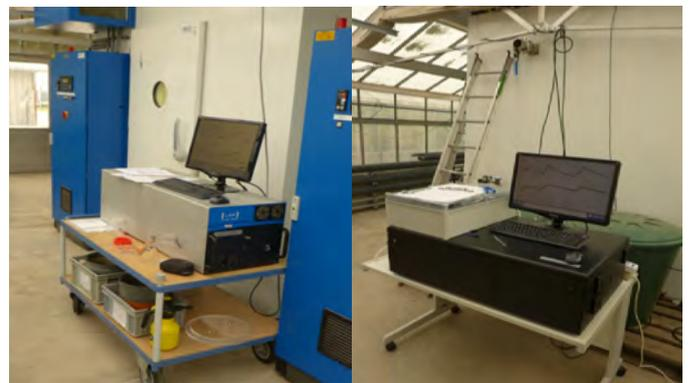
Figure 1. a. Nitrogen-15  $\text{N}_2\text{O}$  laser isotope analyser for screening the efficiency of N process inhibitors in reducing  $\text{N}_2\text{O}$  emission from urea-fertilized applied to lysimeters in growth chamber (left); b. Controlling Carbon-13 enrichment of  $\text{CO}_2$  in the growth chamber during Carbon-13 labelling of maize (right)
