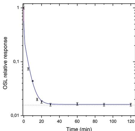
**Figure 8.** OSL relative response of BeO samples optically treated by blue LEDs.
