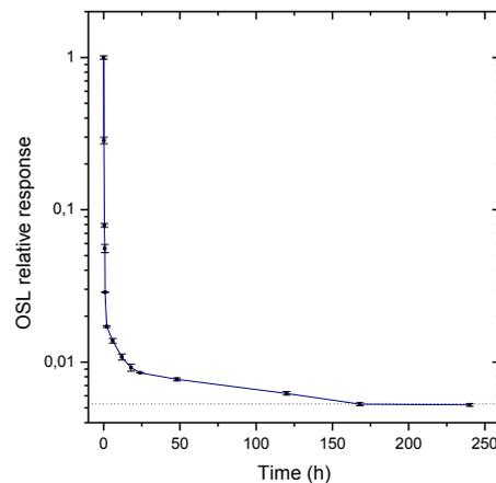
**Figure 7.** OSL relative response of BeO samples irradiated with 1 Gy of absorbed dose ( $^{90}\text{Sr}+^{90}\text{Y}$  source), exposed to different time intervals of the fluorescent system. The dashed line represents the OSL response of non-irradiated samples (OR).
