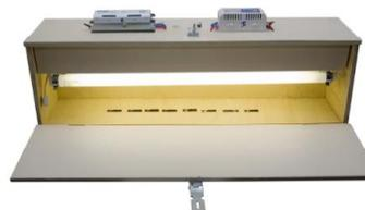
**Figure 4.** Homemade light box with fluorescent lamps [8].
