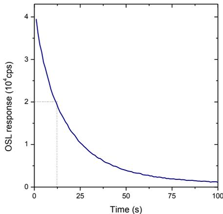
**Figure 5.** OSL decay curve of BeO samples irradiated with 1 Gy of absorbed dose ( $^{90}\text{Sr}+^{90}\text{Y}$  source).
