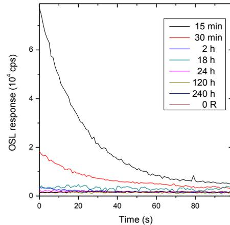
**Figure 6.** OSL decay curves of BeO samples irradiated with 1 Gy of absorbed dose ( $^{90}\text{Sr}+^{90}\text{Y}$  source), exposed to different time interval of the fluorescent system. 0R represents OSL response of non-irradiated samples.
