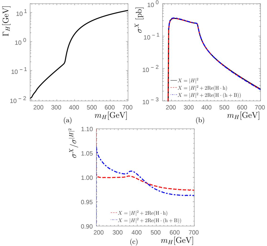
Figure 9: Scenario S1 as a function of the heavy Higgs mass  $m_H$  in GeV showing (a) the Higgs width  $\Gamma_H$  in GeV; (b) the inclusive cross section  $\sigma^X$  in pb within  $m_{ZZ}^I$  and for  $\sqrt{s} = 8$  TeV (black:  $X = |H|^2$ ; red, dashed:  $X = |H|^2 + 2\text{Re}(H \cdot h)$ ; blue, dot-dashed:  $X = |H|^2 + 2\text{Re}(H \cdot h) + 2\text{Re}(H \cdot B)$ ); (c) the relative ratio of cross sections  $\sigma^X / \sigma^{|H|^2}$  within  $m_{ZZ}^I$ .
