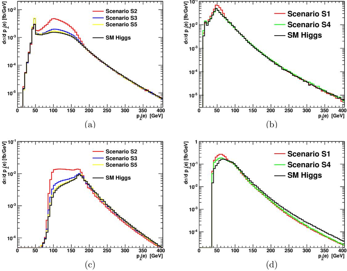
Figure 7: Transverse momentum distribution of the hardest electron (electron or positron) for (a,b)  $gg \rightarrow e^+e^-\mu^+\mu^-$  and for (c,d)  $gg \rightarrow e^+e^-\nu_l\bar{\nu}_l$  at  $\sqrt{s} = 13$  TeV. Due to the different cuts on the invariant mass of the four leptons, the scenarios S2, S3 and S5 (a,c) are plotted separately from S1 and S4 (b,d).
