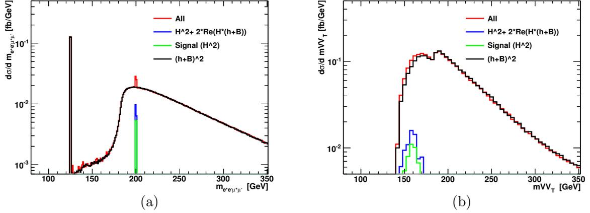
Figure 5: (a) Invariant mass distribution for  $gg \rightarrow e^+e^-\mu^+\mu^-$  and (b) transverse mass distribution for  $gg \rightarrow e^+e^-\nu_l\bar{\nu}_l$  for scenario S4 at  $\sqrt{s} = 13$  TeV.
