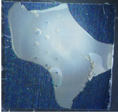
Figure 4: Backside of an ASIC glued with LOCTITE® 3504, removed after curing with UV light guides connected to a mercury arc lamp. The glue layer is broken around three corners of the ASIC and shows additional cracks toward the ASIC centre. No regions of uncured glue were found.
