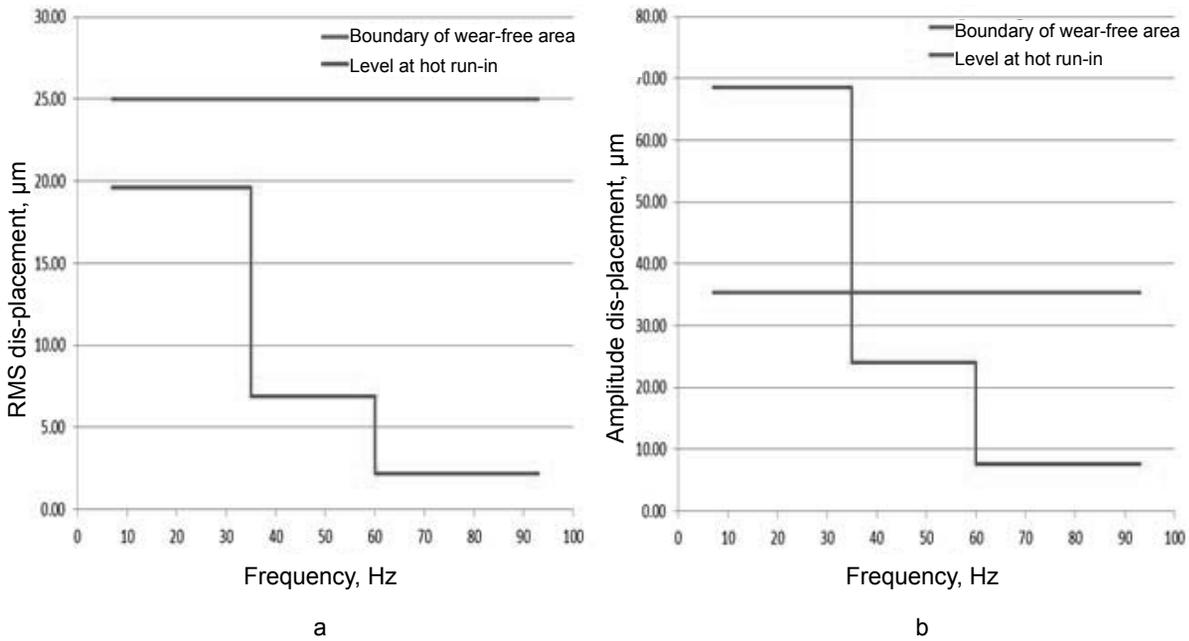
a - Diagram of the level of fuel rod vibrations and boundary of wear-free region (based on RMS values)
