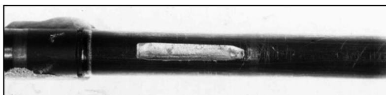
**Figure 3. Worn specimen of fuel rod cladding**
