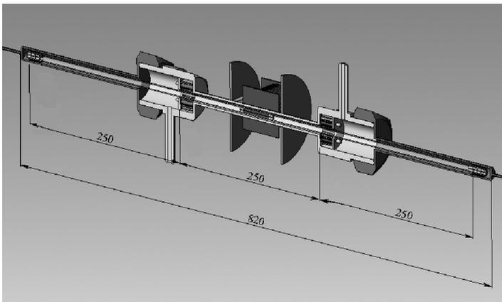
Figure 1. Model to investigate fuel rod cladding fretting wear.
