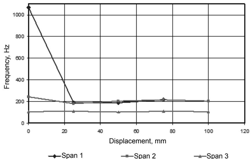
Figure 4. Dependences of natural frequencies of fuel rods on the value of displacement upwards
