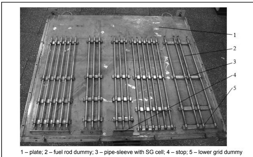
Figure 6. Model for endurance vibration tests of the FA lower part fragments
