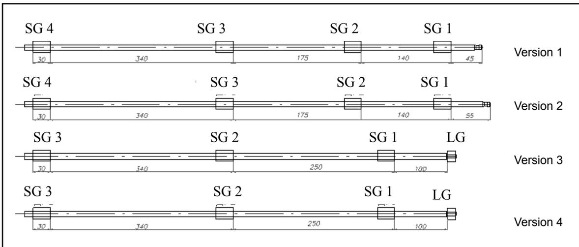
Figure 5. Fragments for vibration endurance tests
