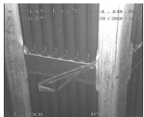
FA № ЕД01044 on 3-d SG tearing of the top part of the rim
