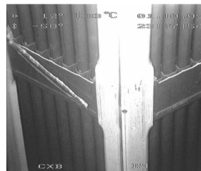
FA № ЖЕД0817 on 4-th SG tearing of the top part of the rim
