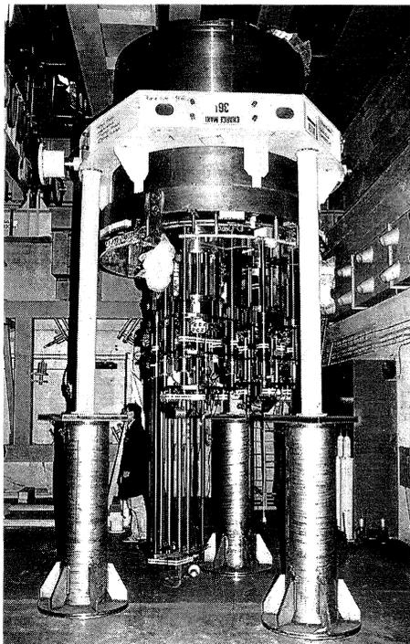
a technique which allows the mandrel to be cooled by circulating liquid helium rather than by immersing the coil. This also avoids micro-movements which cause local overheating. High magnetic fields of 4 to 5 Tesla can therefore be achieved over a substantial distance (2 to 3 metres).
