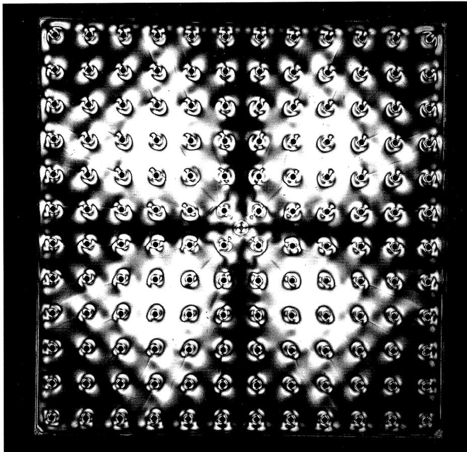
type of sampling calorimeter with wavelength-shifting fibre readout developed recently by IHEP with INR (Moscow), where "perforated" scintillator tiles (see cover photograph, April 1993) with many precision-positioned holes.
