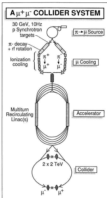
Possible muon collider, as envisaged by Dave Neuffer and Bob Palmer, with the muon beams (from the decay of pions) controlled by ionization cooling before injection into a multiturn recirculating linac arrangement, à la CEBAF, before finally being prepared for collision.
