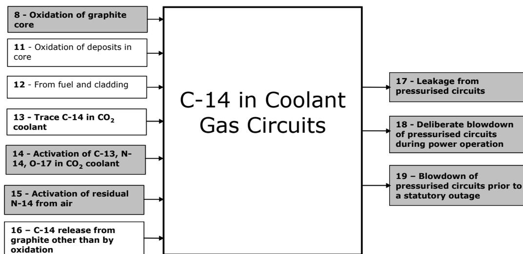
FIG. 5. Schematic representation of abbreviated gas coolant circuits model showing C-14 inputs and outputs highlighted in grey.
