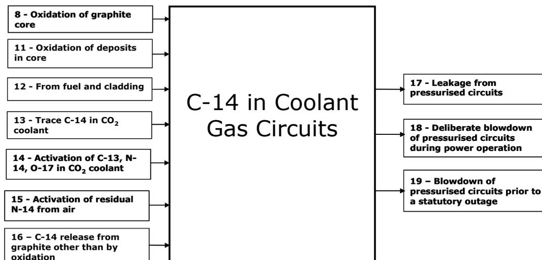
FIG. 3. Schematic representation of coolant gas circuits model showing C-14 inputs and outputs.
