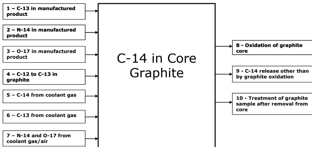
FIG. 2. Schematic representation of graphite core model showing C-14 inputs and outputs.
