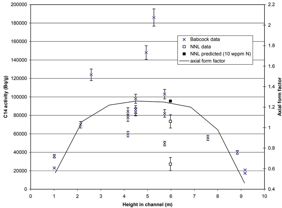
FIG. 6. Axial variation in C-14 activity in the Wylfa cores compared with activation modelling prediction
