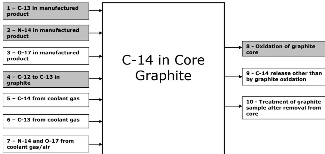
FIG. 4. Schematic representation of abbreviated graphite core model showing C-14 inputs and outputs highlighted in grey.
