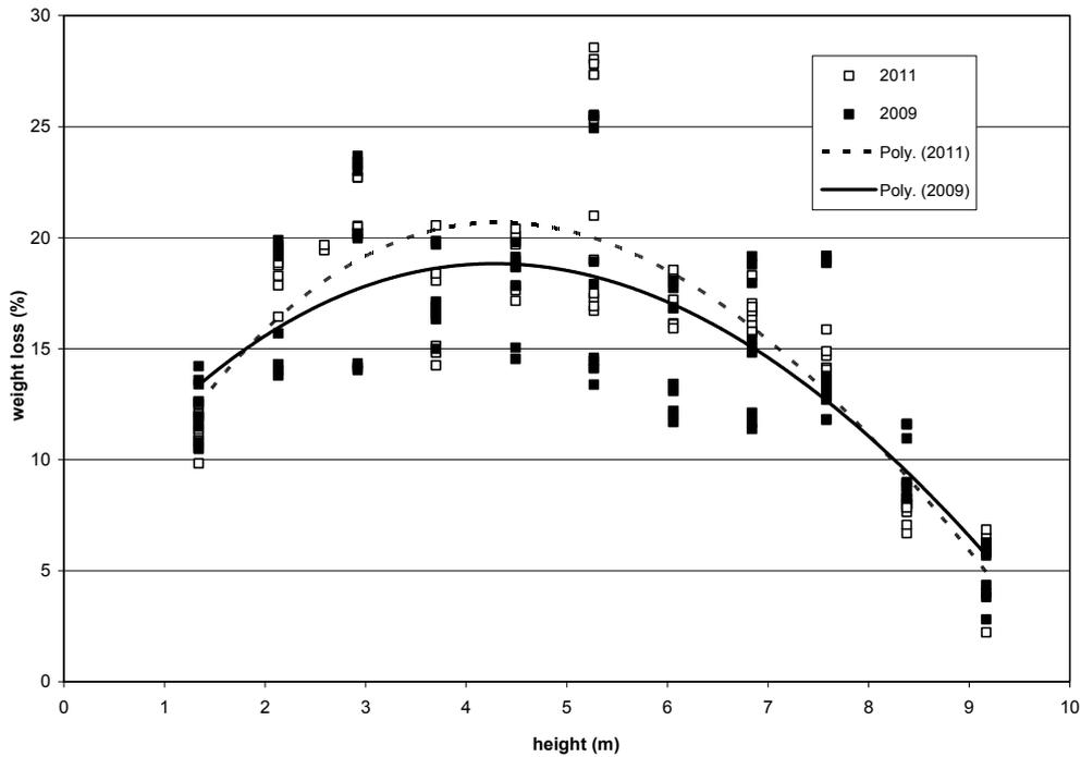
FIG.7 Interstitial channel graphite weight loss data for the Wylfa Reactor 1 core at 2009 and 2011
