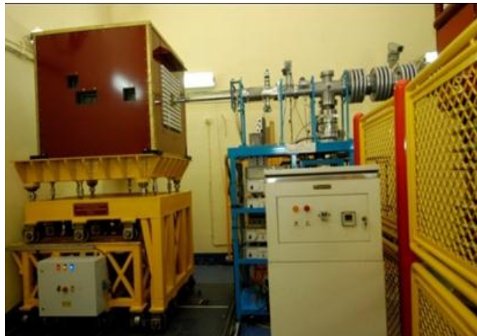
Fig.2. Subcritical core being coupled to neutron generator
