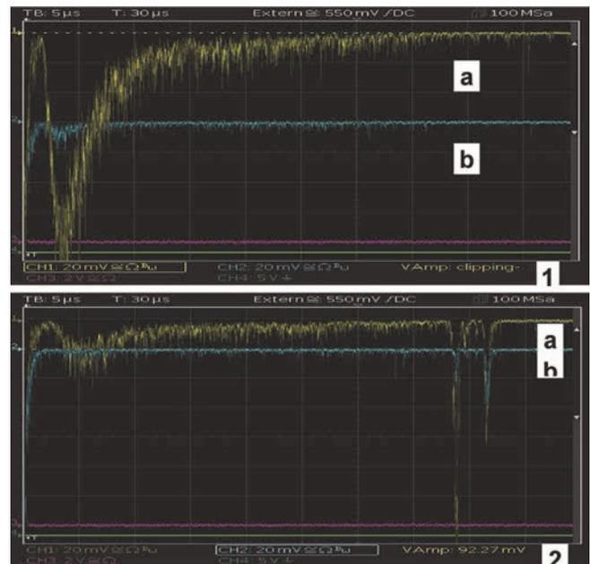
Figure 6. The Scattering from Atmosphere and Clouds received signal oscillograms. a – parallel with laser beam polarization channel, b – crossed with laser beam polarization channel (Horizontal - 5us/div; Vertical -20mV/div).
