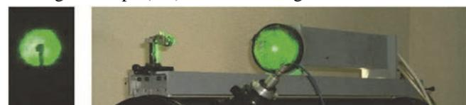
**Figure 2.** The Laser Emitter, including the beam expander in operation mounted on the RT (in the right) and the Laser Emitter output beam-spot on the distance of 2 meters (in the left).
