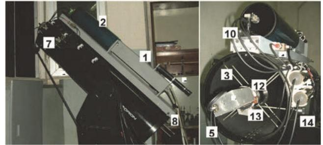
Figure 4. The LIDAR system. 1 - The Laser; 2 - Laser Beam Expander; 3 - RT; 4 - PS; 5 - Signal optical fiber bundles; 6 - Optical filter boxes; 7 - PMTs; 8 - LE alignment platform; 9 - Aiming optics; 10 - Triggering and output energy control optical fiber bundles; 11 - Triggering photodiode; 12 - PS alignment mount; 13 - Stepper motor with Play-free Gear; 14 - RT mirror focus finder.
