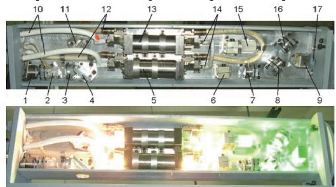
**Figure 1.** The Laser construction (left): 1 - Convex mirror, 2 - Electro optical Q-Switch, 3 - Diaphragm, 4 - Output polarizer, 5 - laser oscillator pump chamber, 6 - Quarter wave-plate, 7 - Concave mirror, 8 and 16 - Two wavelength mirrors, 9 - Glan prism, 10 - Flash-lamp driver cables, 11 - mirror, 12 - Cooling system pipes, 13 - Laser amplifier pump chamber, 14 - Flash-lamps, 15 - SHG, 17 - Hole for the output beam. The Laser in operation (right).
