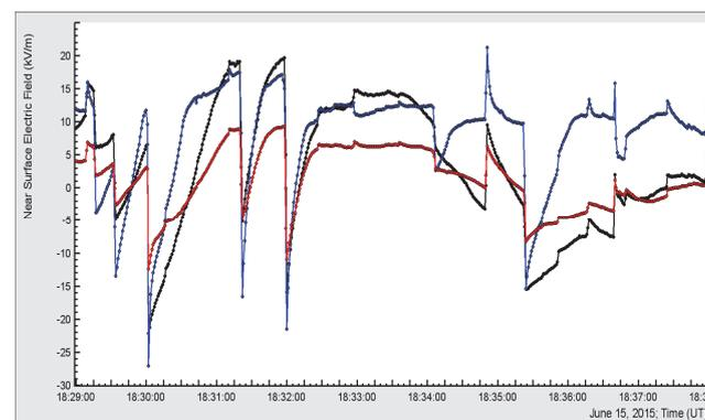
Figure 3. Disturbances of near-surface electrostatic field measured by the network of EFM-100 type electric mills at Mt. Aragats on June 15 2015 (zoomed version of 10 minutes from Fig.2)
