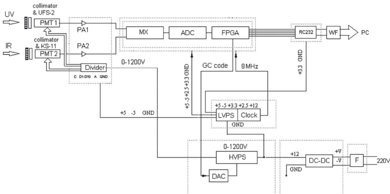
Figure 1. Diagram of the electronics of the DUVIR device.
