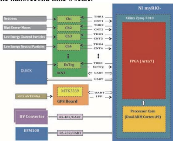
Figure 10. National Instruments myRIO board for the synchronized detection of particle fluxes, UV and IR radiation and disturbances of the near-surface electrostatic field.
