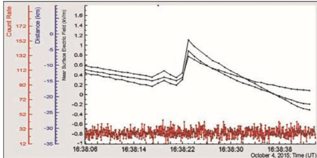
Figure 5. Negative lightning detected by the network of electric mills and particle count rate (at the bottom)
