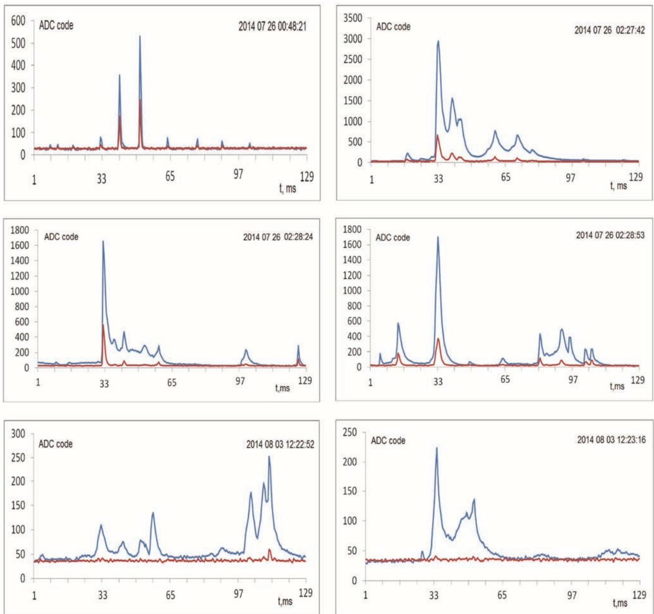
Figure 9. Examples of the waveforms of lightning flashes recorded on board of the "Vernov" satellite.
