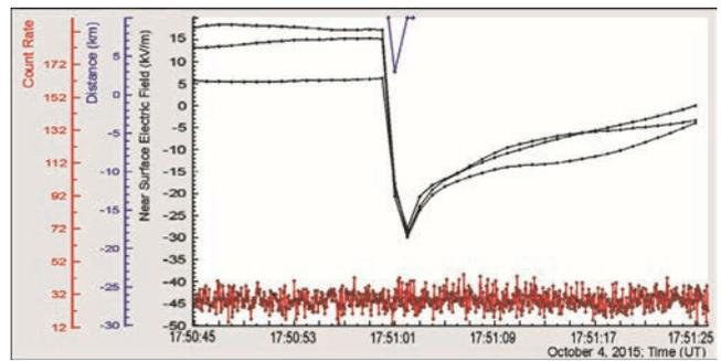
Figure 6. Positive nearby lightning detected by the network of electric mills and particle count rate (at the bottom)
