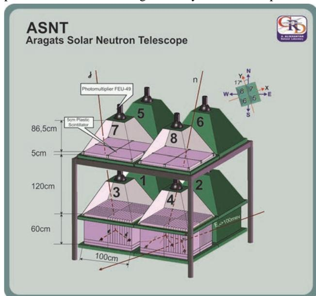
Figure 1. Setup of the Aragats Solar Neutron Telescope (ASNT)
