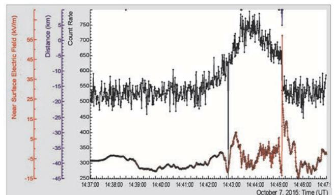
Figure 5. TGE abruptly terminated by the negative lightning; in the bottom are shown electric field disturbances detected by the electric mill EFM-100; in the middle – 1-sec time series of count rate of 3 cm thick outdoor plastic scintillator, on the top – distance to lightning; Lightning occurred at 14:45:07 coinciding with decline of particle flux by 14.4%.
