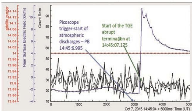
**Figure 6.** Five seconds of 50 ms time series of all 3 layers of the STAND1 detector (located near SKL hall) before and after sharp decline of particle flux at 14:45:07.225. The flux decline coincides with an abrupt increase (100 ms rise time) of the near-surface electrostatic field. 14 GPS satellites participate in the precise time synchronization.
