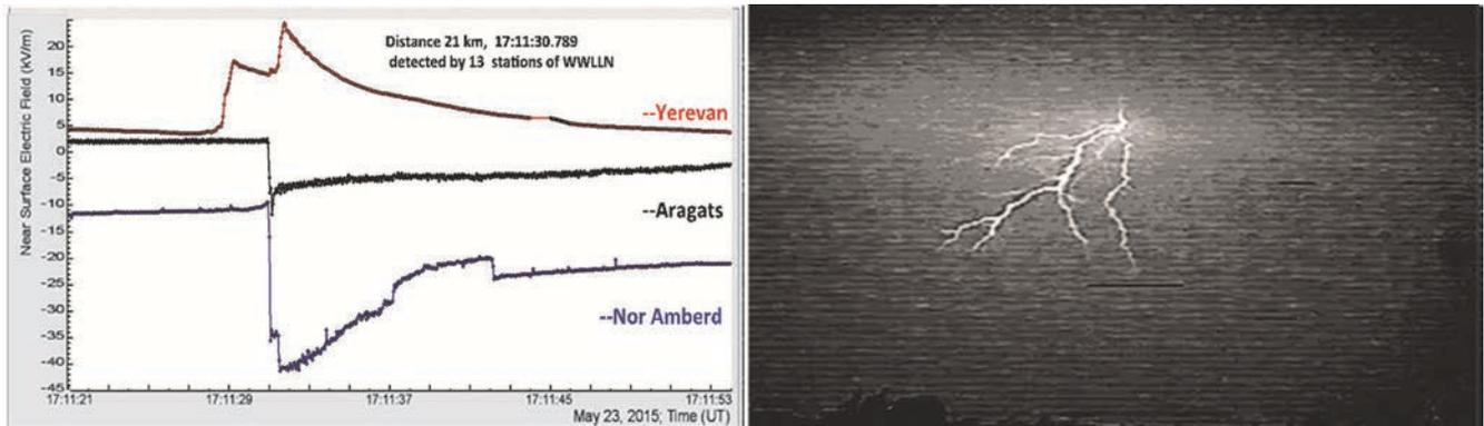
Figure 9. The disturbances of the near-surface electric field due to intracloud lightning shown on the photograph shot at Burakan village in direction of Mt. Ararat. On the top are shown the measurements of the near-surface electric field performed by the EFM-100 electric mills located at Aragats, Nor Amberd and Yerevan. Polarity reversal of electrostatic field change for the negative IC flash is apparent.
