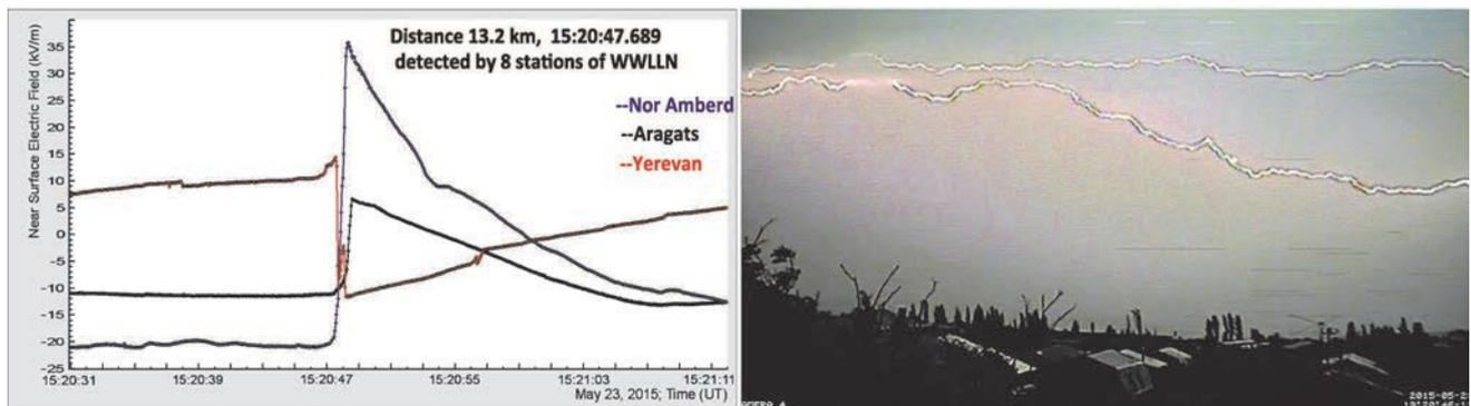
Figure 8. The disturbances of the near-surface electric field due to intracloud lightning shown on the photograph shot at Burakan village in direction of Mt. Ararat. On the top are shown the measurements of the near-surface electric field performed by the EFM-100 electric mills located at Aragats, Nor Amberd and Yerevan. Polarity reversal of electrostatic field change for the negative IC flash is apparent.
