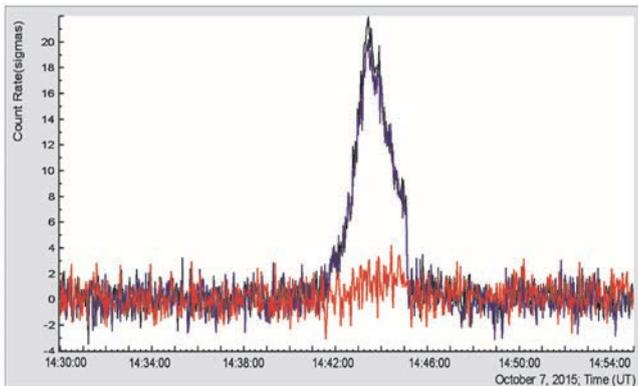
Figure 3. TGE as seen in the p-values of the two-second time series of the ASNT detector; black time series – total flux; blue time series – flux with veto on near-vertical charged particles; red time series – high energy particles with energies greater than 20 MeV.
