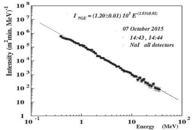
Figure 4. Differential energy spectrum of the TGE measured by the NaI spectrometer with energy threshold 0.4 MeV
