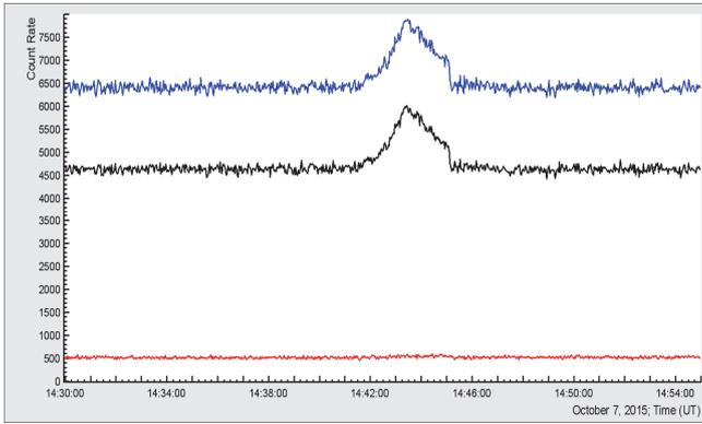
Figure 2. TGE seen in the two-second time series of the ASNT detector; blue time series – total flux; black time series – flux with veto on near-vertical charged particles; red time series – high energy particles with energies greater than 20 MeV.
