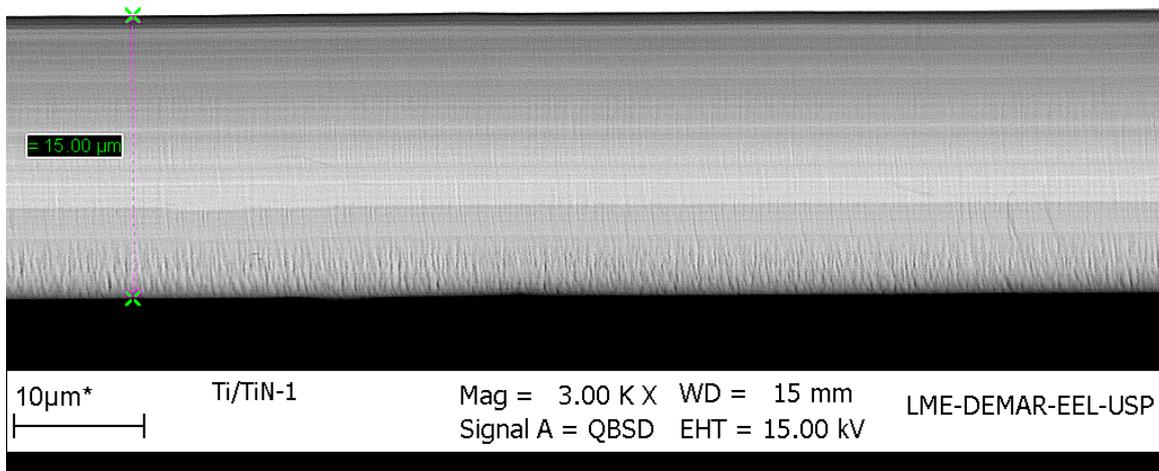
Figure 5- TiN substrates after deposition by EB-PVD at 600°C for 25 minutes.
