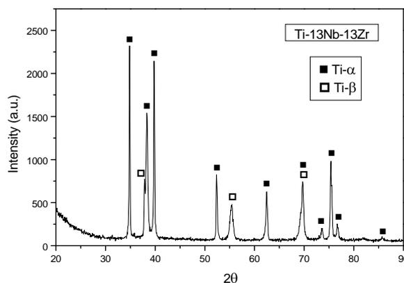
Figure 3- X-ray spectra of Ti-13Nb-13Zr substrate sintered at 1400 °C.
