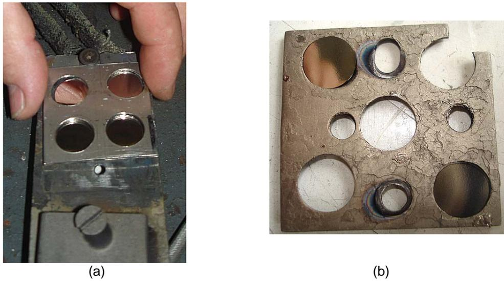
Figure 4- (a) Ti-13Nb-13Zr substrates mounting for EB-PVD evaporation; (b) substrates after deposition at 350°C for 25 minutes.
