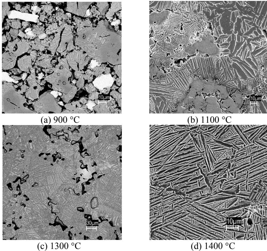
Figure 1- Microstructural evolution of the BE-Ti-13Nb-13Zr during sintering. All samples were sintered at the nominal temperature for 1 h and heating rate equal to 20 °C min<sup>-1</sup>.
