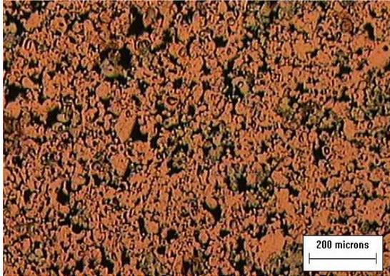
Figure 1 Optical micrograph of the alloy Cu-1%Ni-1%Al, cold compact (1000kPa) and sintered at 650°C for 1200s
