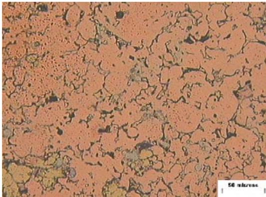
Fig.2- Optical micrograph of the alloy Cu-1%Ni-0.5%Al, cold compact (1000kPa) and sintered at 780°C for 5400s.
