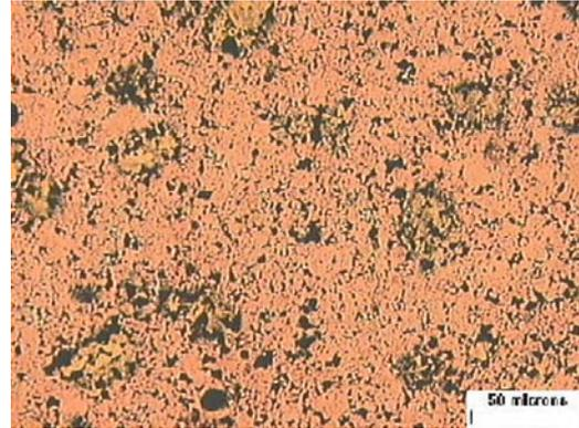
Fig.3- Optical micrograph of the alloy Cu-1%Ni-0.5%Al, cold compact (1000kPa) and sintered at 780°C for 5400s
