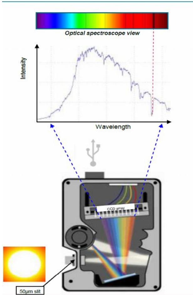
**Figure 1: Concept of spectrometer**
