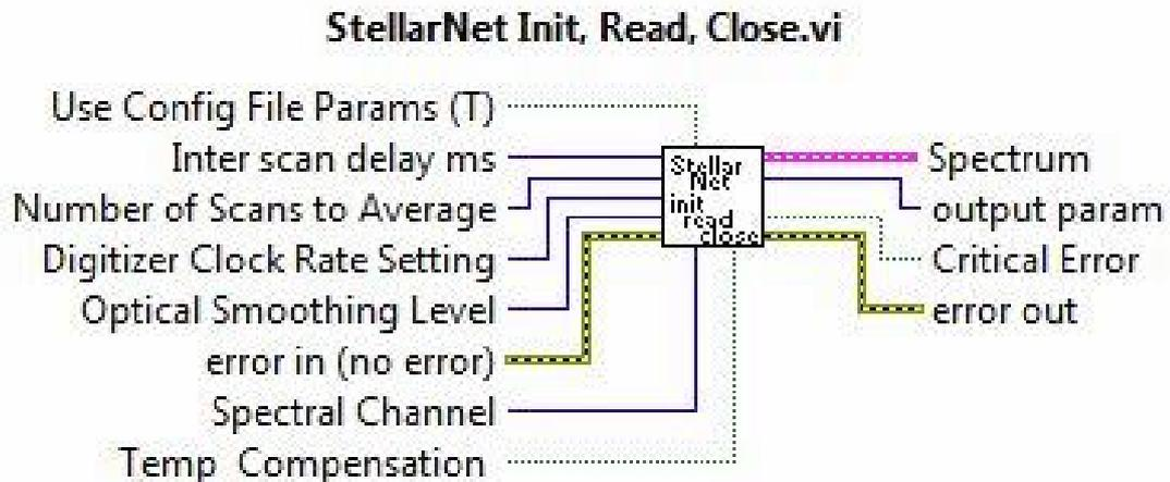
**Figure 2: LabVIEW driver to read data from StellarNet USB spectrometer**
