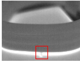
Figure 4: The red square shows the location of visual formation of defect
