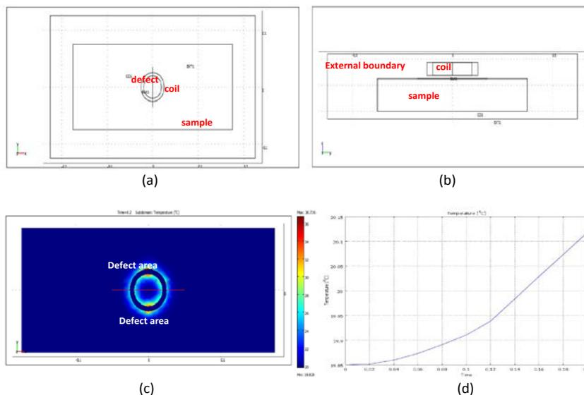
Figure 5: The simulation of COMSOL FEM Multiphysics.
