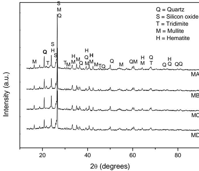
**Figure 1.** X Ray patterns of ceramic materials, sinterized under the temperature of 1150<sup>0</sup>C.
