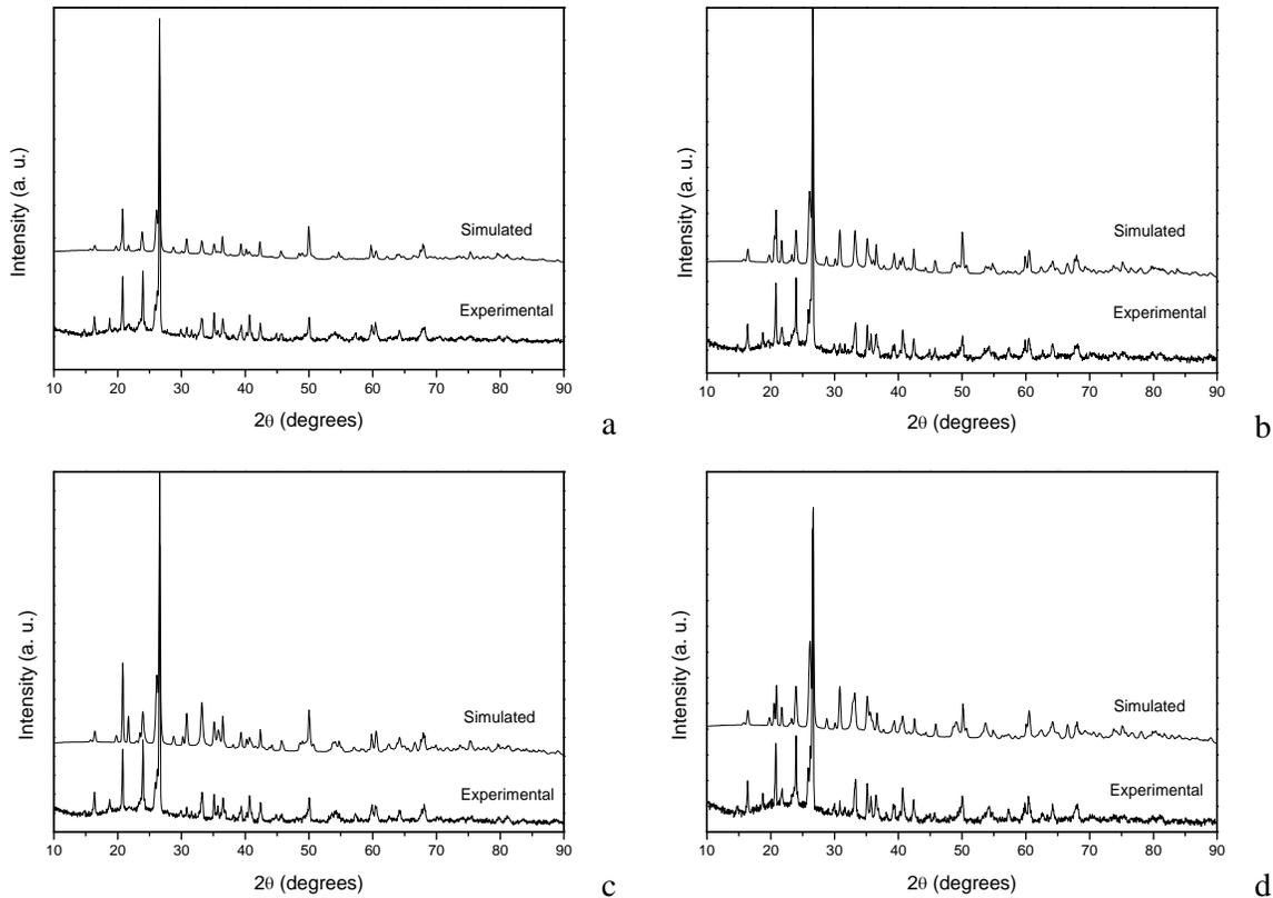
**Figure 2.** Materials MA, MB, MC and MD patterns, experimental and simulated by the Rietveld Method.
