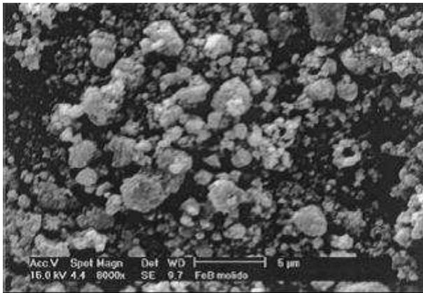
Fig. 3. Micrograph of Fe/B powder by SEM, after 36 h mechanical alloying.
