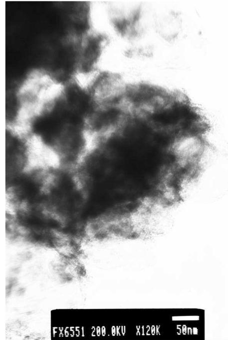
Fig. 4. Micrograph of Fe/B powder by TEM, after 36 h mechanical alloying.
