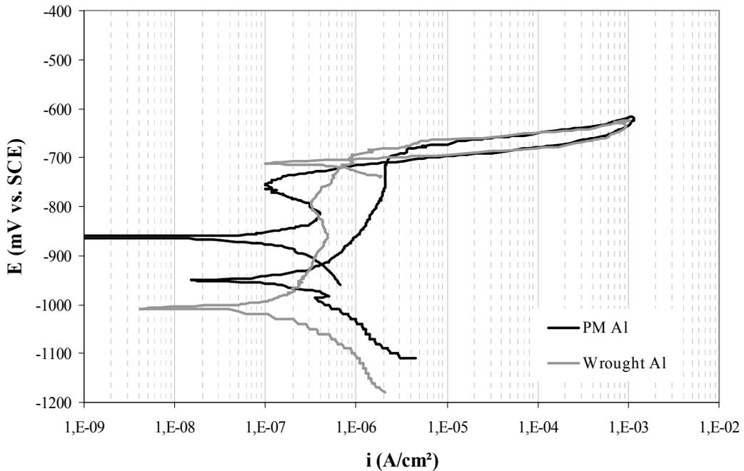
Fig. 5. Cyclic anodic polarization curves of a wrought aluminium and a plain aluminium.
