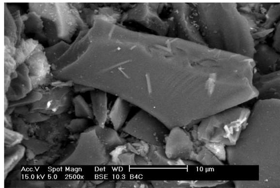
Fig. 2.  $B_4C$  powder used as reinforcement in AMCs.
