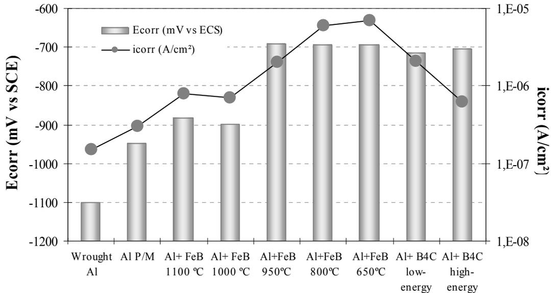
Fig. 8. E<sub>corr</sub> and i<sub>corr</sub> values in deaerated NaCl 0.1 M of all studied materials.
