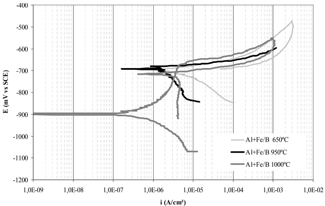
Fig. 6. Cyclic anodic polarization curves of aluminium with 20% Fe/B sintered at 1000, 950 and 650 °C.
