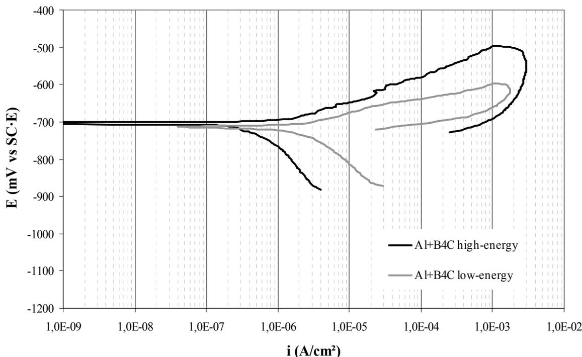
Fig. 7. Cyclic anodic polarization curves of aluminium with 10% B<sub>4</sub>C for both mixing powders' conditions.
