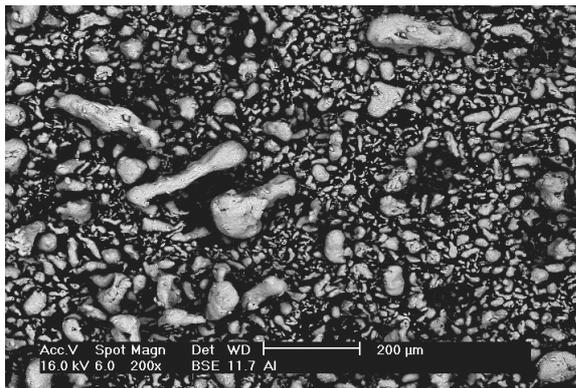
Fig. 1. Aluminium powder used as base material.
