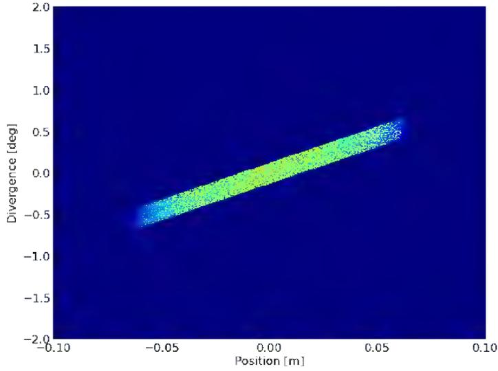
**Figure 2** Phase space of the neutron beam at the exit of the beam tube in planned configuration of VENUS, as simulated using McStas. The maximum divergence is about  $\pm 2^\circ$ .
