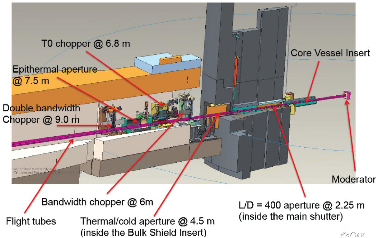
**Figure 1** Schematic drawing of the VENUS's front-end optics (the beam tube) between the neutron moderator and the experimental hutch.
