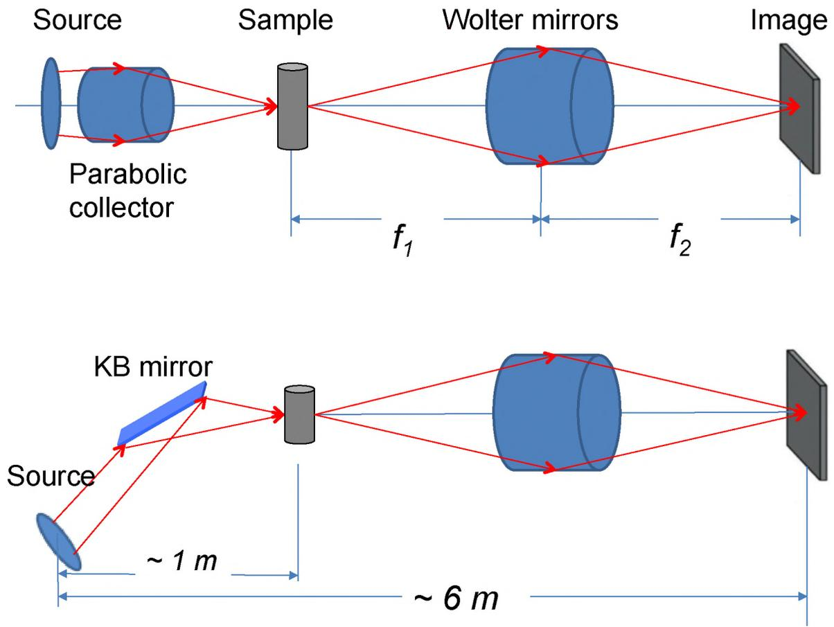
**Figure 3.** Schematic drawings of two possible focusing devices for creating a diverging beam at the sample position.
