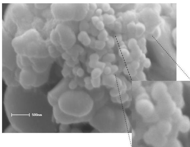
**Figura 4:** SEM image of the sample calcined at 550°C.
