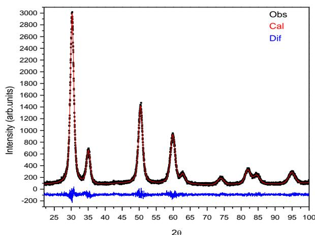
**Figure 1:** Rietveld refinement plot for the powder calcined at  $550^\circ\text{C}$ : in red is the calculated diffraction pattern, in black is the observed diffraction pattern and in blue is the difference among observed and calculated diffraction pattern.
