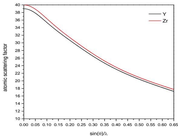
**Figure 3:** Atomic scattering factor for atoms Zr and Y,  $\text{CuK}\alpha$  Radiation.
