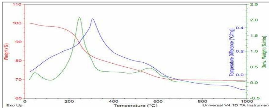
Figure 5 Thermal analysis of organophilic bentonite Chiqui Gómez
