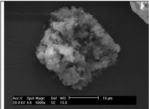
Figure 3 A crystalline stacked grain of bentonite.
