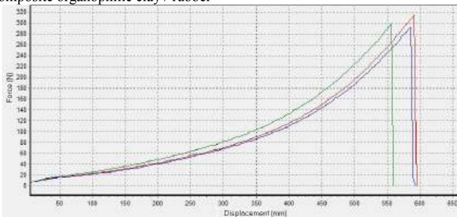
Figure 5 Stress-strain curves of a rubber nanocomposite with 10 per of organophilic clay. The same composition with 40 per of carbon-black show tensile strength lesser than 11 MPa. The results on three samples were 22,4 ; 19,5 and 17,5 MPa respectively. This
