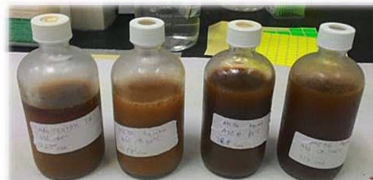
Figure 5: Water extracts of F. deltoidea leaf samples using ASE at variable temperature
