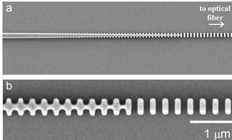
Fig.1: *Subwavelength grating fibre-chip coupler for silicon waveguides.*
